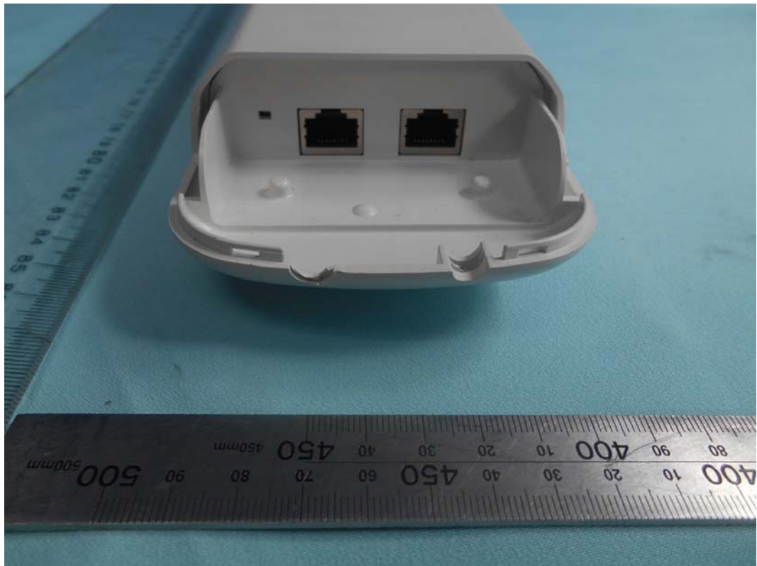
FIGURE 3 INTELLIGENT WIRELESS TRANSMISSION EQUIPMENT (M/N: TB5E) PORTS
