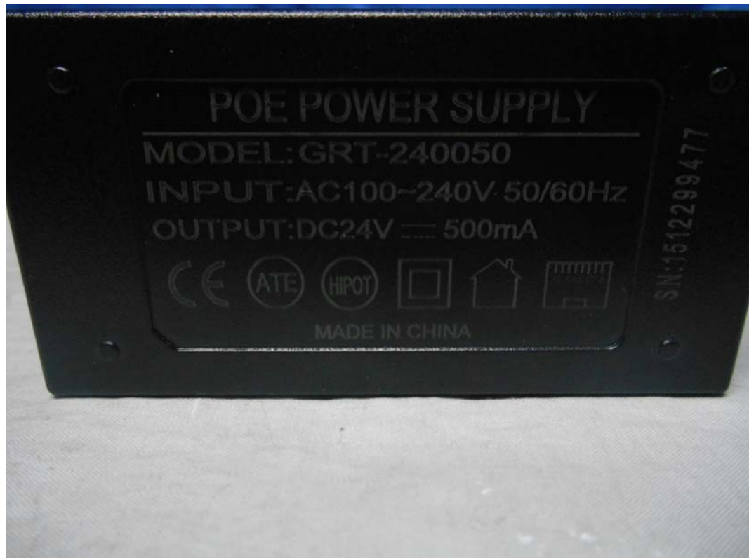
FIGURE 14 INTELLIGENT WIRELESS TRANSMISSION EQUIPMENT (M/N: TB5E) POE POWER ADAPTER LABEL
