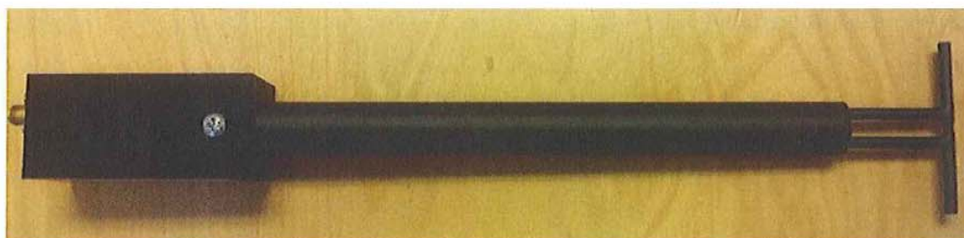
Figure 1 – MVG COMOSAR Validation Dipole
