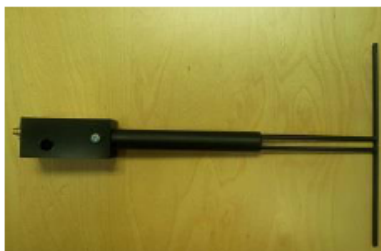
Figure 1 – MVG COMOSAR Validation Dipole
