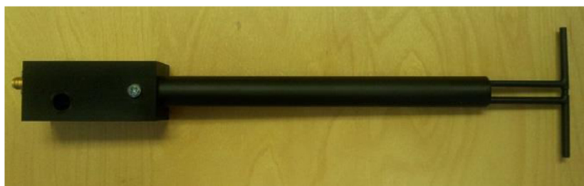
Figure 1 – MVG COMOSAR Validation Dipole
