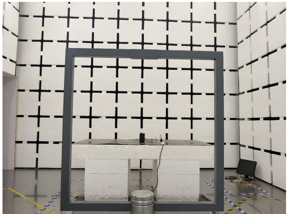
Radiation Emission Test Setup (Below 30MHz)
