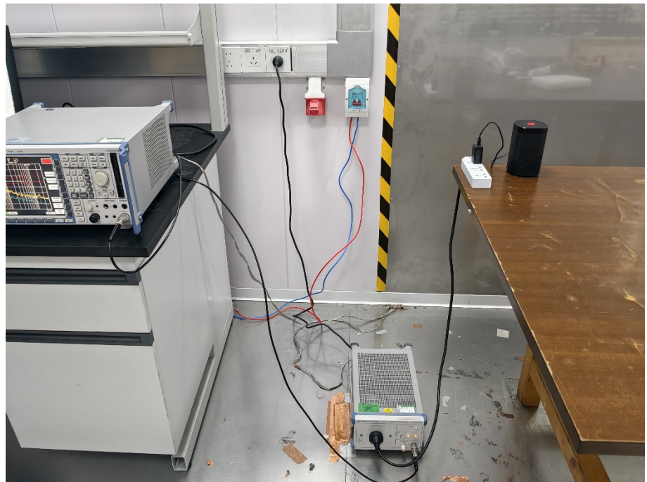
Conducted Emission Test Setup
