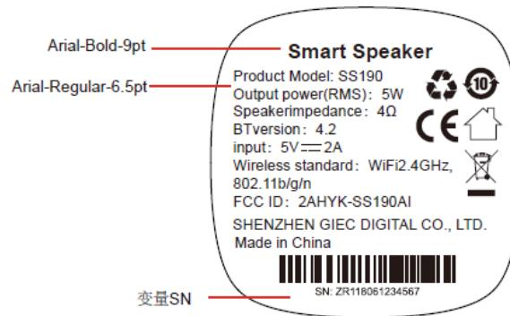
Specifications: The label shall be securely affixed to a permanently attached part of the device, in a location where it is visible or easily accessible to the user, and shall not be readily detachable. The label shall be sufficiently durable to remain fully legible and intact on the device in all normal conditions of use throughout the device's expected lifetime.
