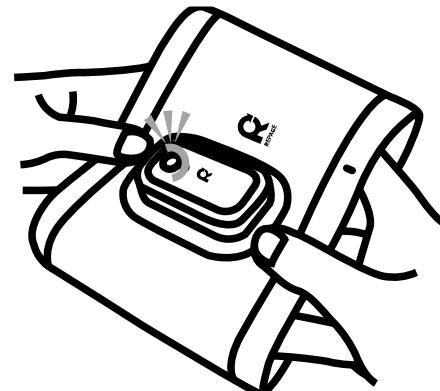
1. Insert the REPACE into the holder according to the shape of the sensor holes.
