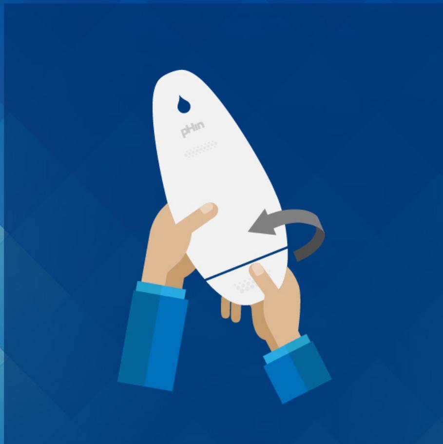
Twist end cap clockwise, then pull down to remove
