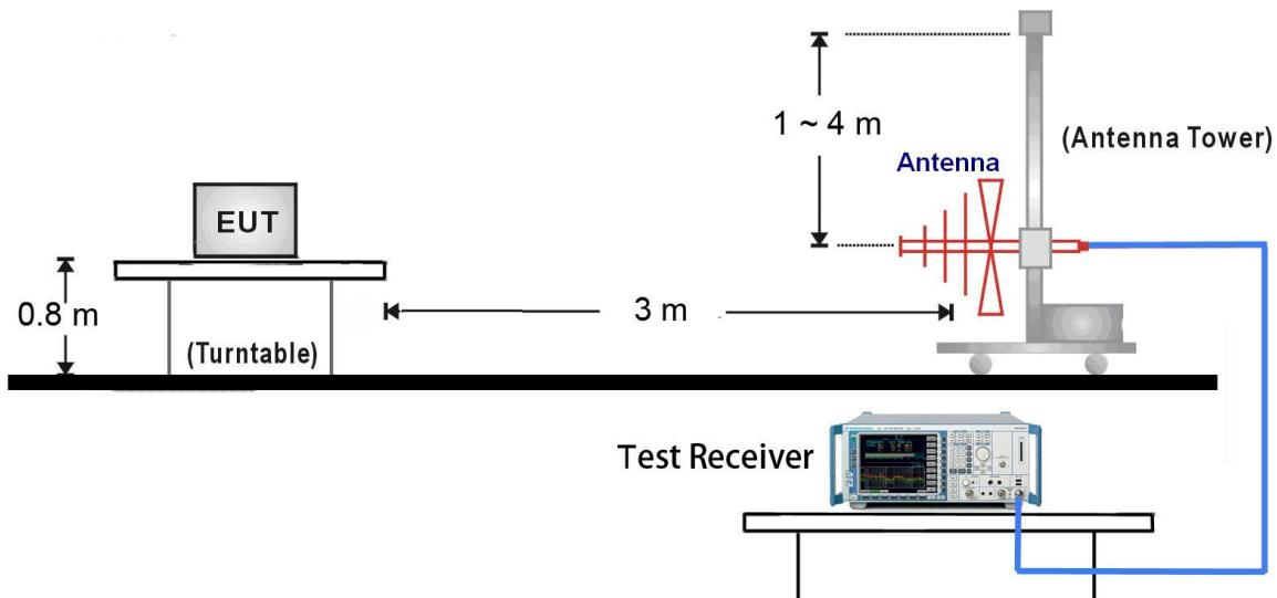
1GHz ~ 25GHz Test Setup:
