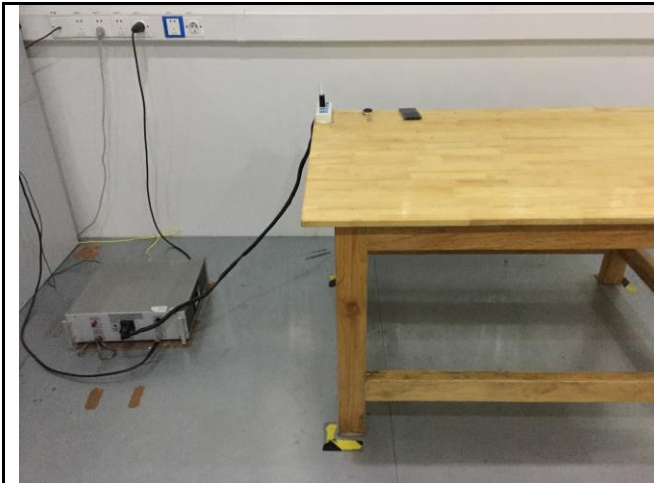
Conducted Emissions Test Setup Front View
