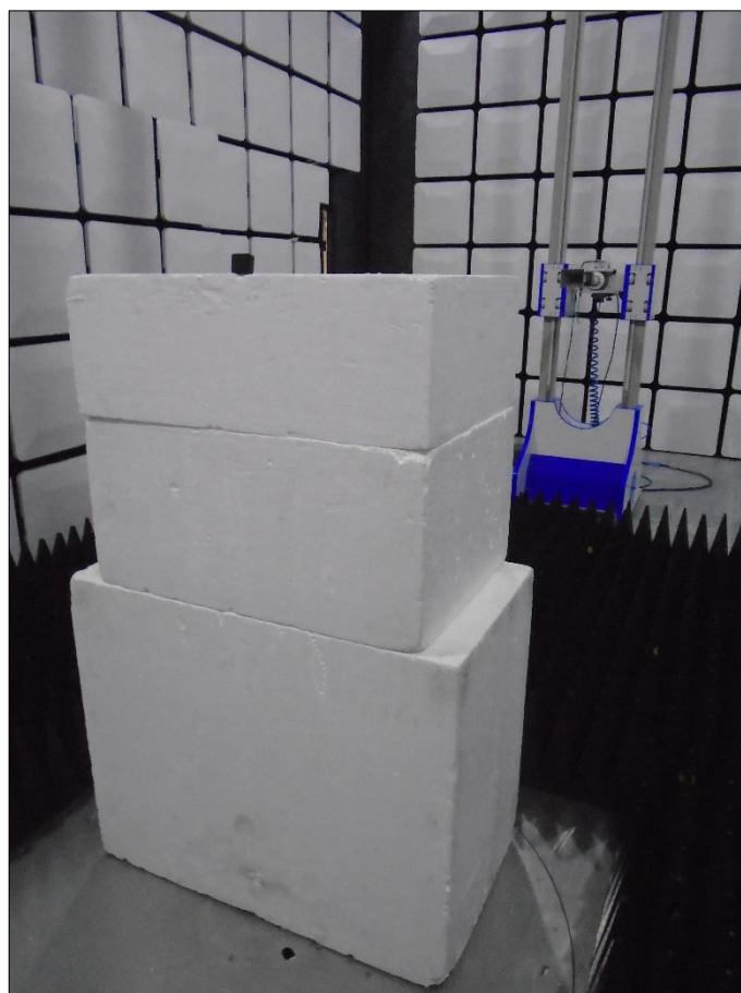
Figure 65 - Test Setup - 1 GHz to 18 GHz - Z Orientation
