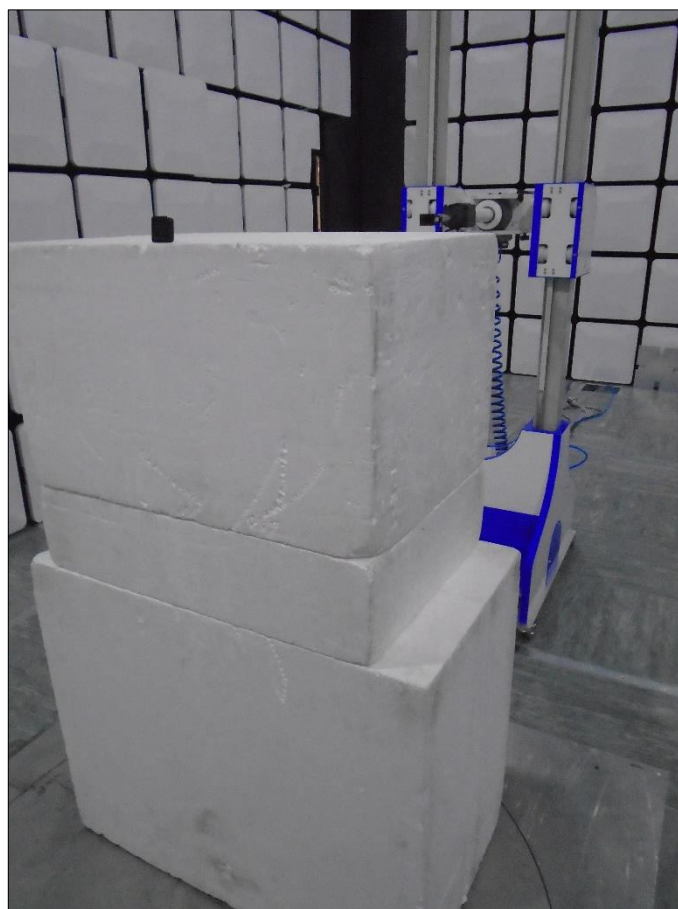
Figure 67 - Test Setup - 18 GHz to 25 GHz - Y Orientation
