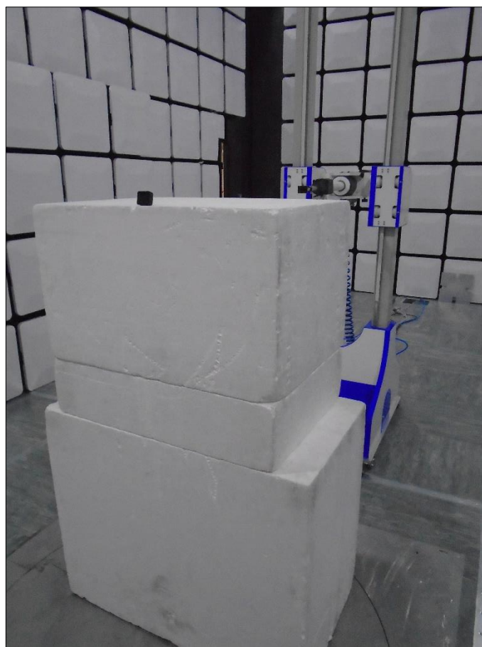
Figure 68 - Test Setup - 18 GHz to 25 GHz - Z Orientation
