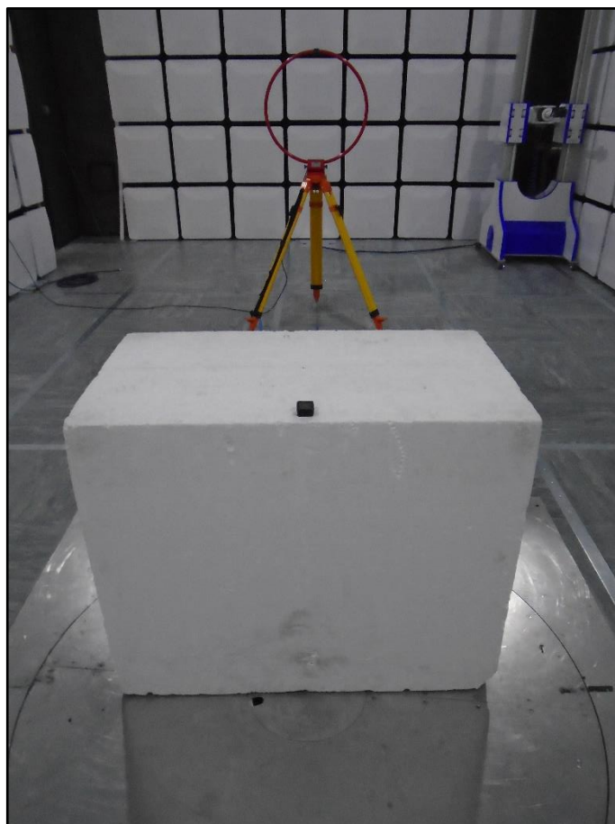
Figure 15 – Test Setup – 9 kHz to 30 MHz, Orientation X
