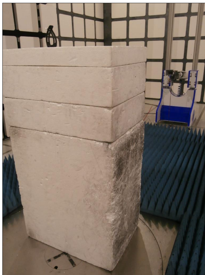
Figure 59 - Test Setup - 8 GHz to 18 GHz
