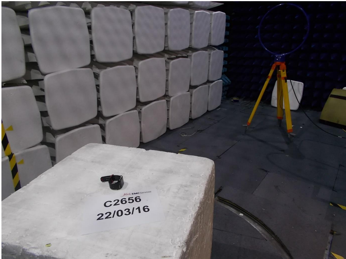
Chamber measurement 9kHz to 30MHz
