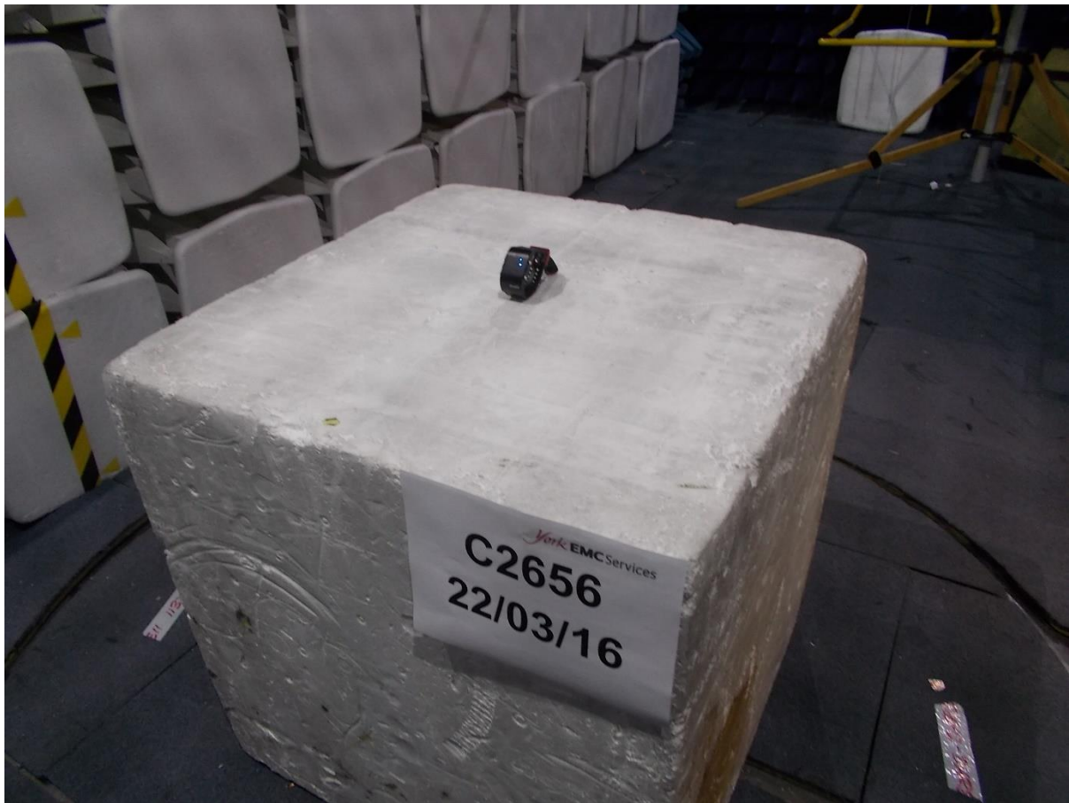
Chamber measurement 30MHz to 1GHz
