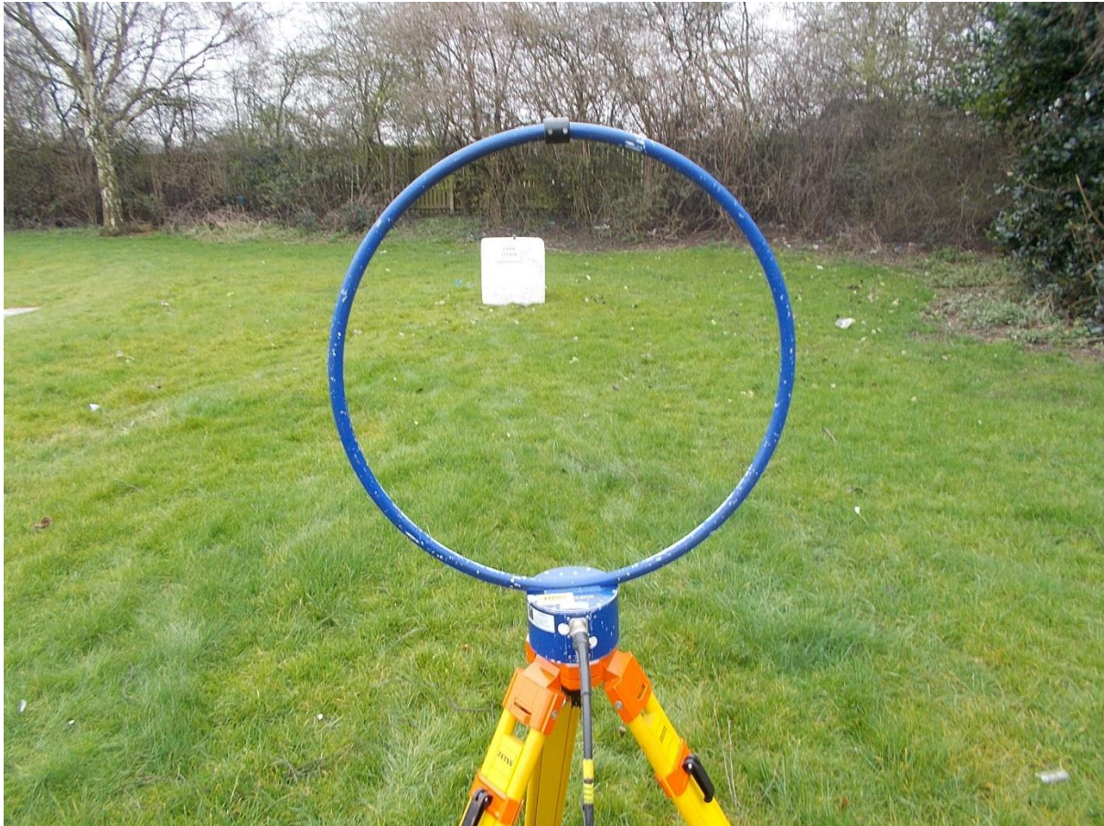
Final radiated emissions 9kHz to 30MHz
