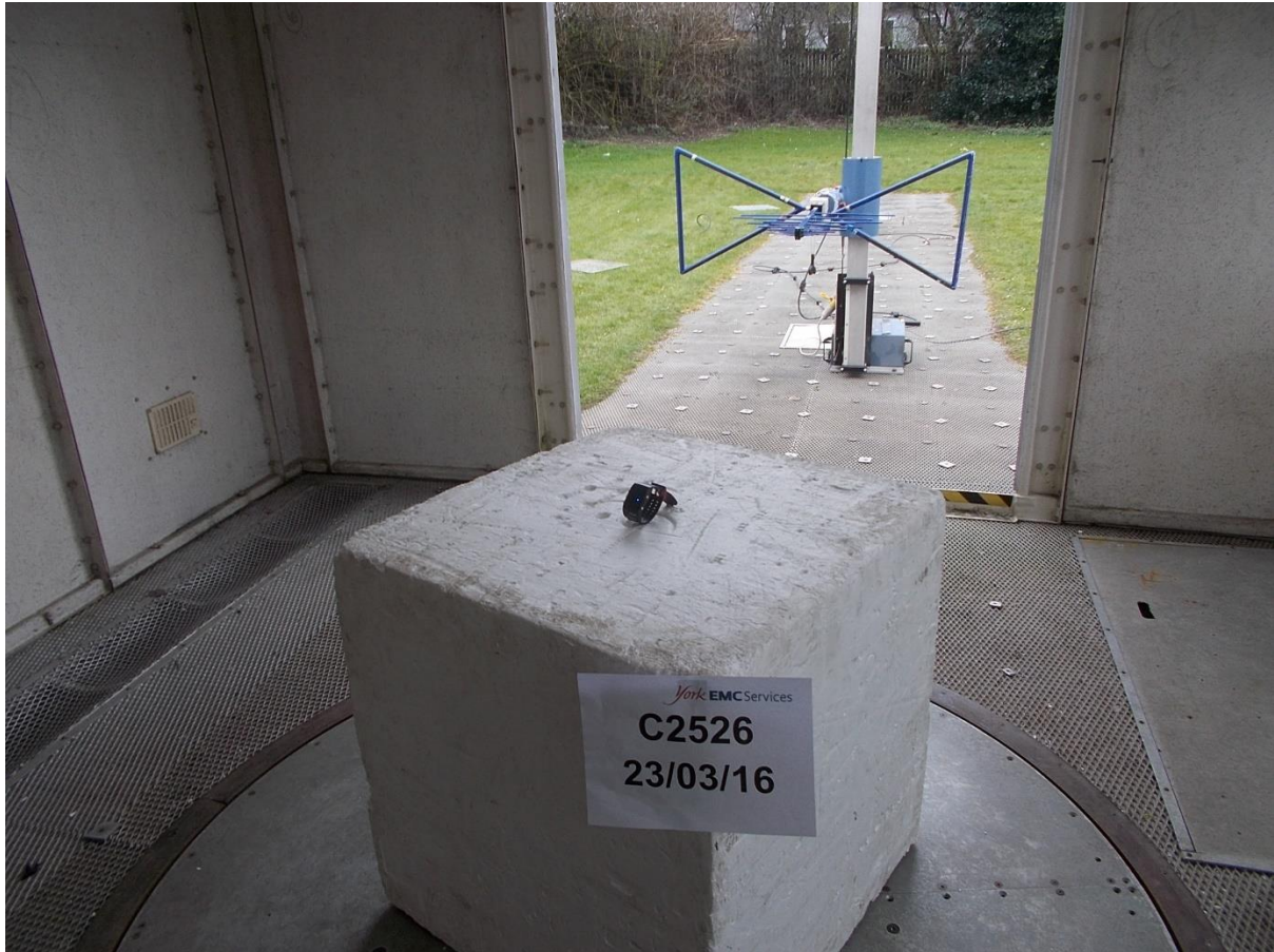
Final radiated emissions test 30MHz to 1GHz – OATS
