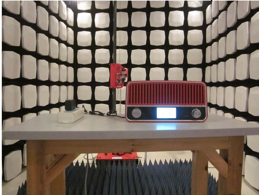
Measurement of Radiated Emission Test Set Up
