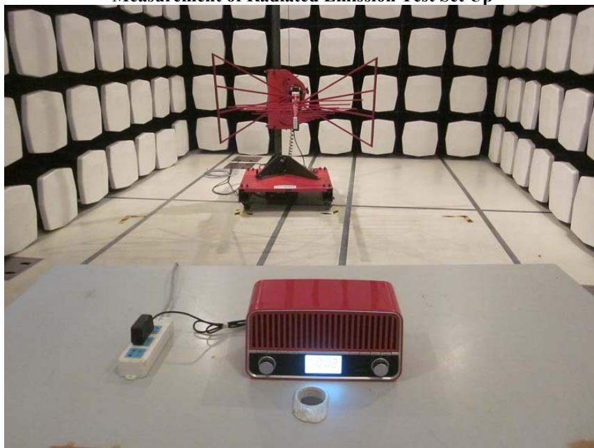
Measurement of Radiated Emission Test Set Up
