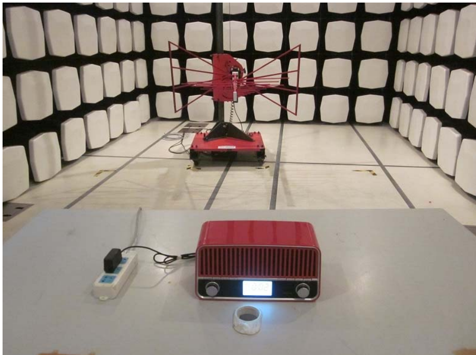
Measurement of Radiated Emission Test Set Up
