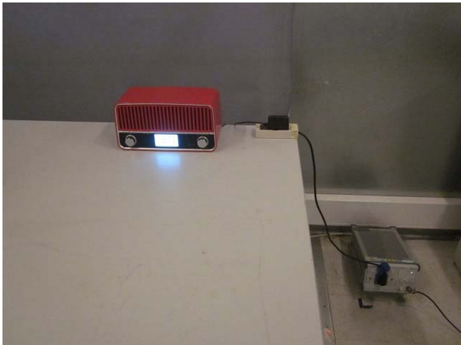
Measurement of Conducted Emission Test Set Up
