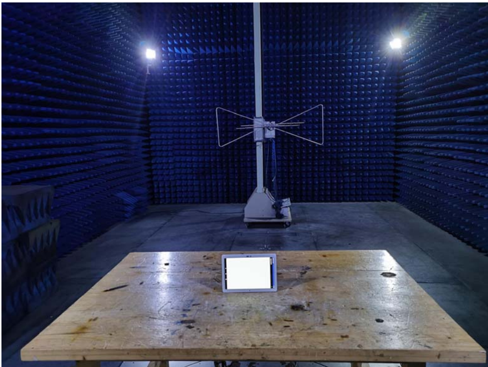
Photo of Radiated Emission Measurement (Below 1G)
