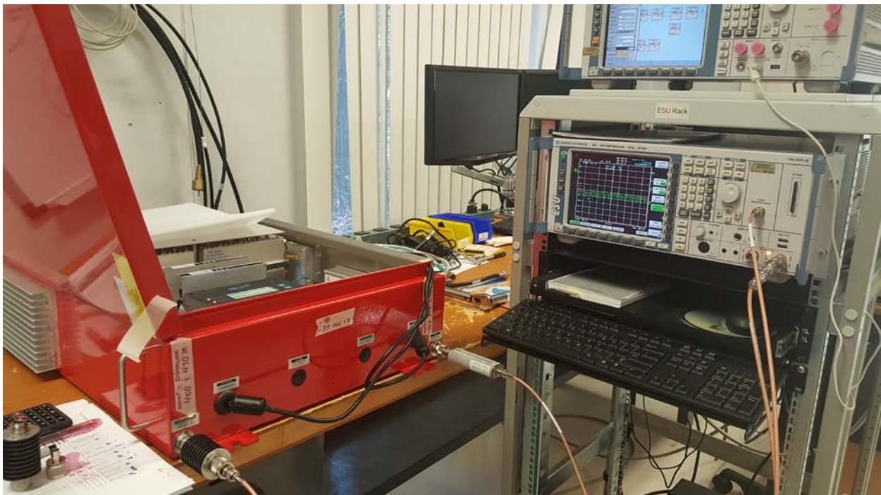
**FIELD STRENGTH SPURIOUS EMISSIONS – TABLE SETUP, REAR**
