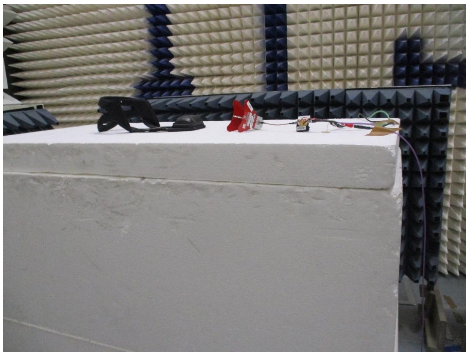
Figure 0-6 Radiated Spurious Emissions Test Setup Above 18 GHz
