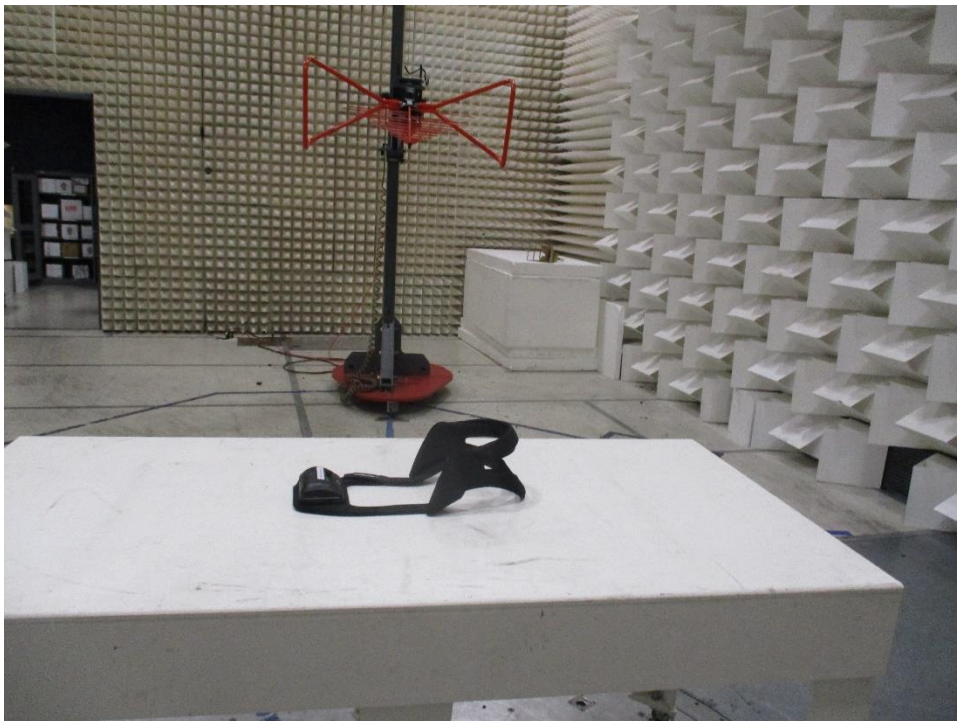
Figure 0-2 Radiated Spurious Emissions Test Setup 30 MHz-1 GHz Battery Mode Back Side
