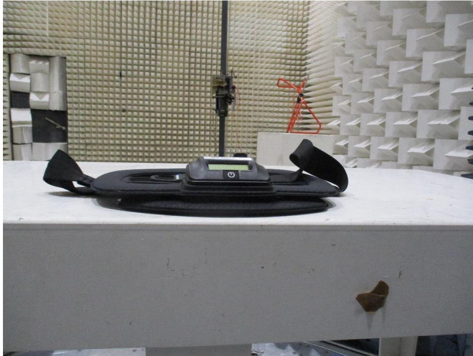
Figure 0-35 Radiated Emissions Test Setup Above 1 GHz Battery Mode Back Side
