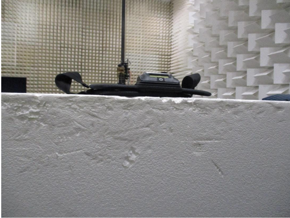
Figure 0-33 Radiated Spurious Emissions Test Setup 1 GHz-18 GHz Battery Mode Back Side
