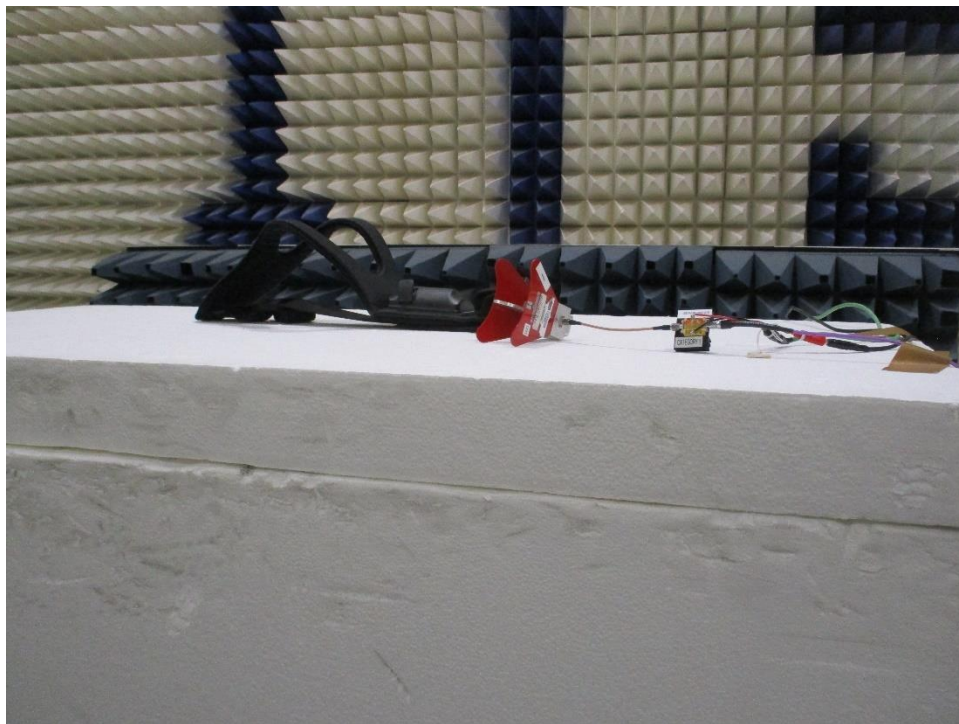
Figure 0-20 Radiated Spurious Emissions Test Setup Above 18 GHz
