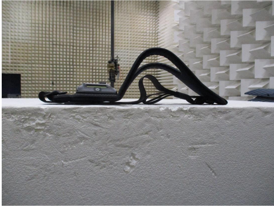
Figure 0-19 Radiated Spurious Emissions Test Setup 1 GHz-18 GHz Battery Mode Back Side
