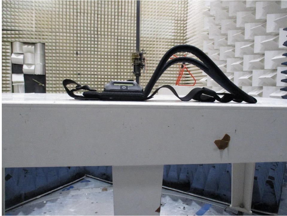
Figure 0-21 Radiated Emissions Test Setup Above 1 GHz Battery Mode Back Side
