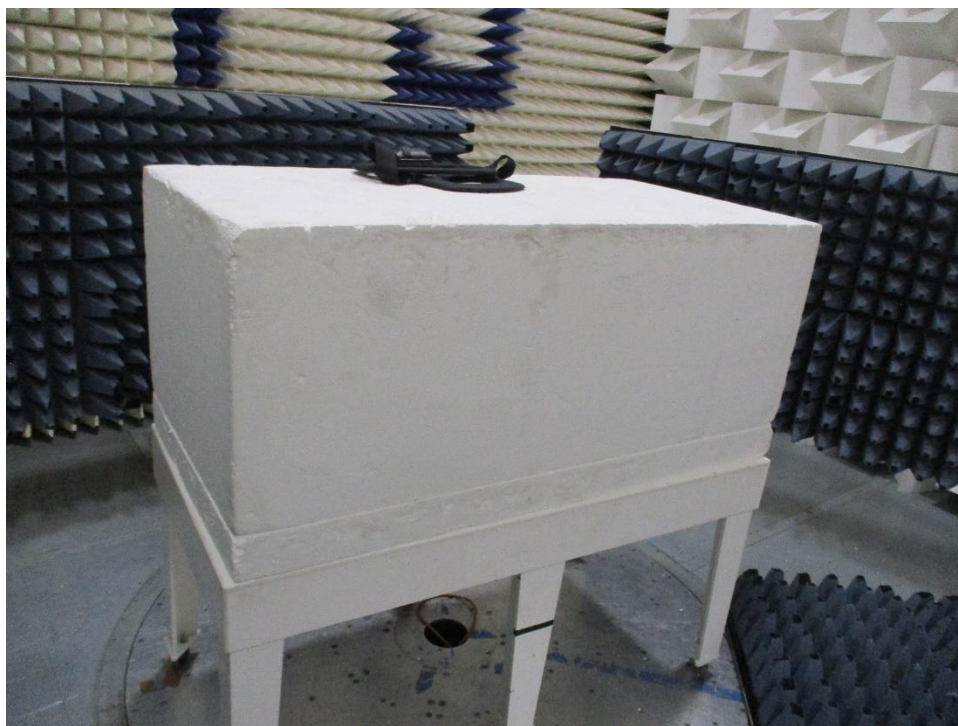
Figure 0-32 Radiated Spurious Emissions Test Setup 1 GHz-18 GHz Battery Mode Front Side
