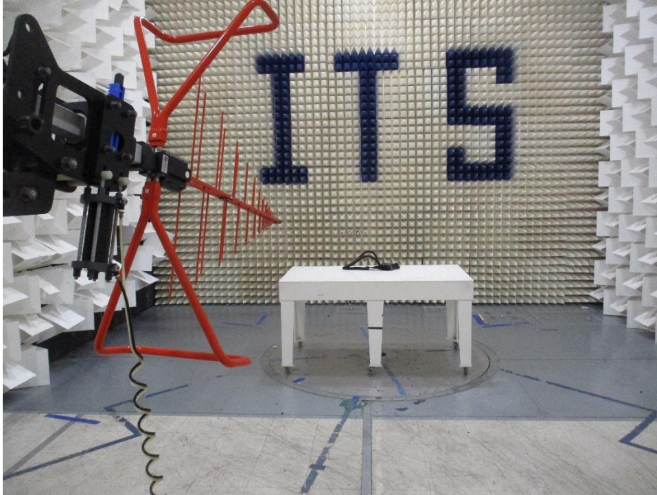
Figure 0-15 Radiated Spurious Emissions Test Setup 30 MHz-1 GHz Battery Mode Front Side
