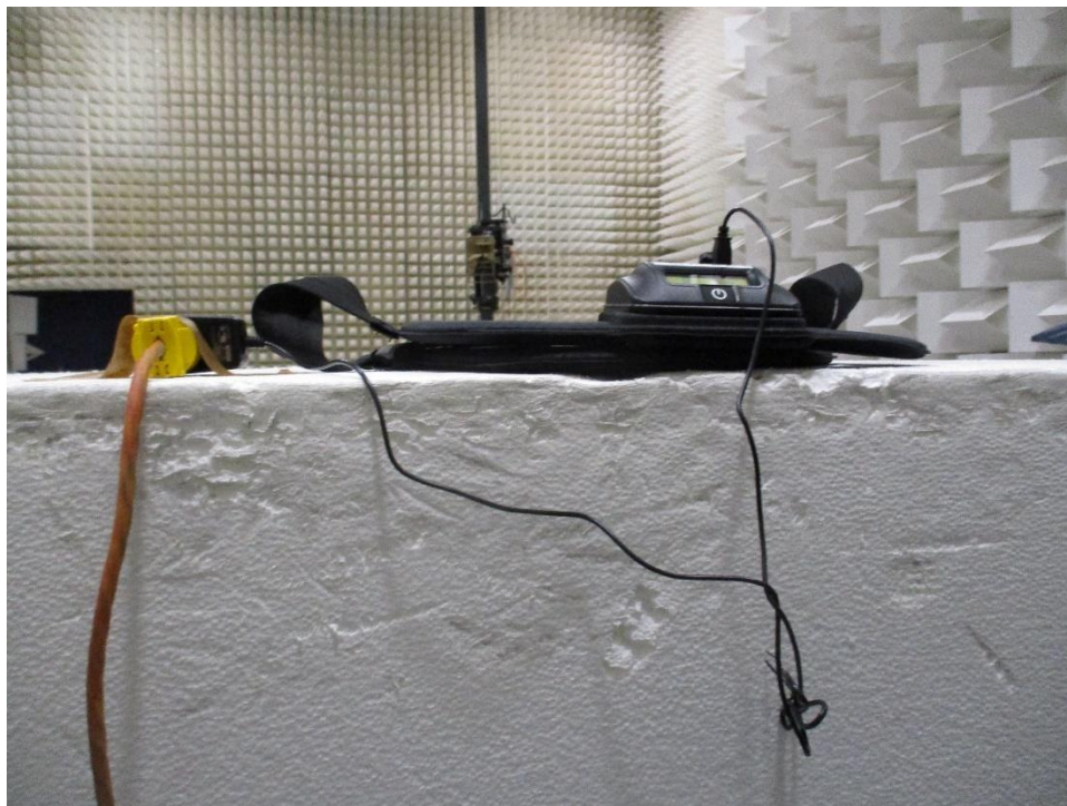
Figure 0-39 Radiated Spurious Emissions Test Setup 1 GHz-18 GHz Charging Mode Back Side
