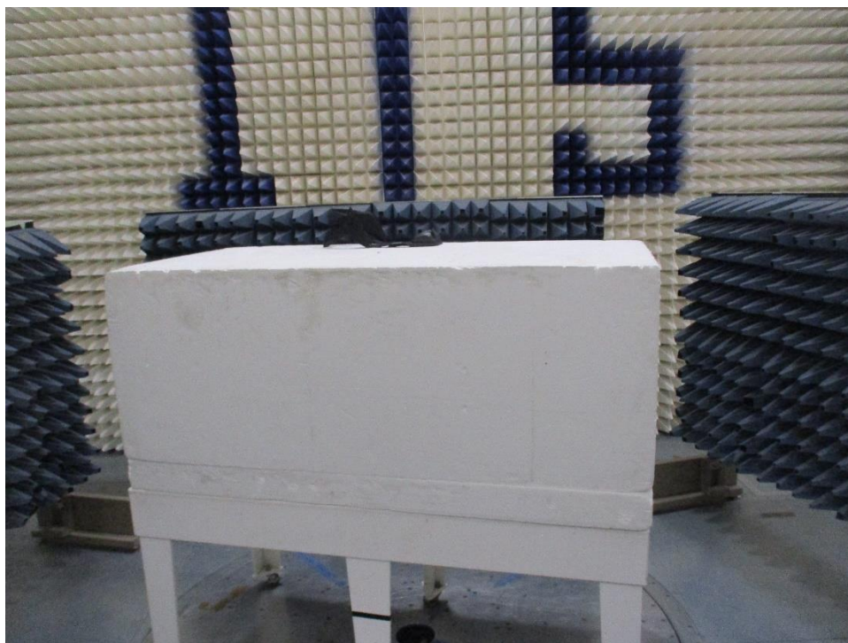
Figure 0-4 Radiated Spurious Emissions Test Setup 1 GHz-18 GHz Battery Mode Front Side
