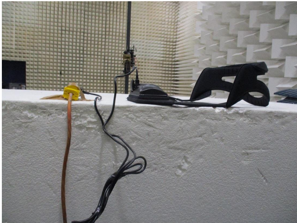
Figure 0-12 Radiated Spurious Emissions Test Setup 1 GHz-18 GHz Charging Mode Back Side
