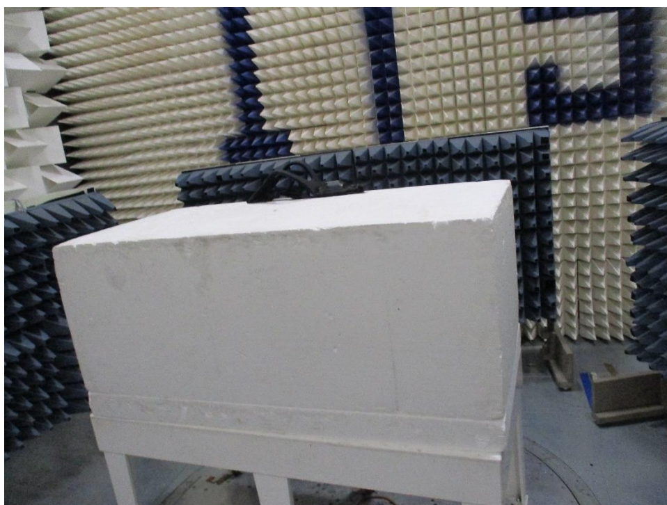
Figure 0-18 Radiated Spurious Emissions Test Setup 1 GHz-18 GHz Battery Mode Front Side
