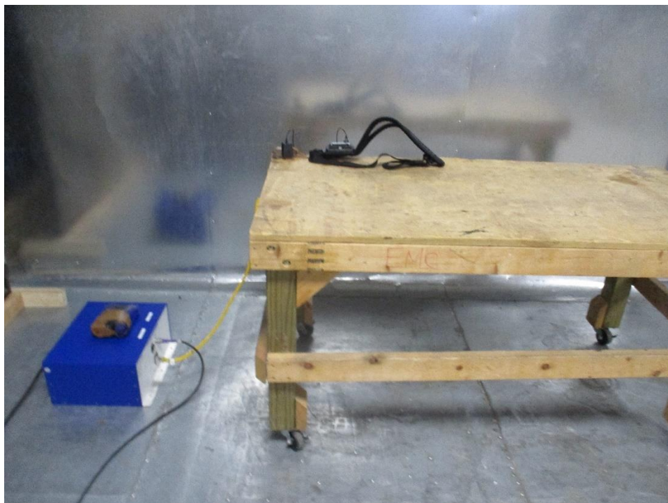
Figure 0-28 Conducted Emissions Test Setup
