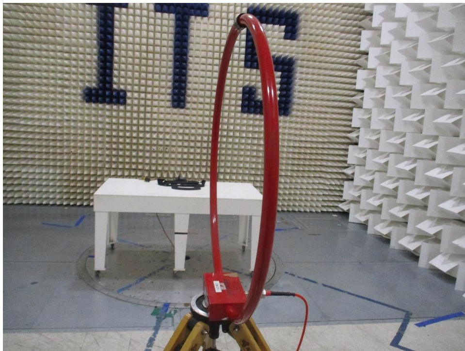
Figure 0-38 Radiated Spurious Emissions Test Setup 9 kHz-30 MHz Charging Mode
