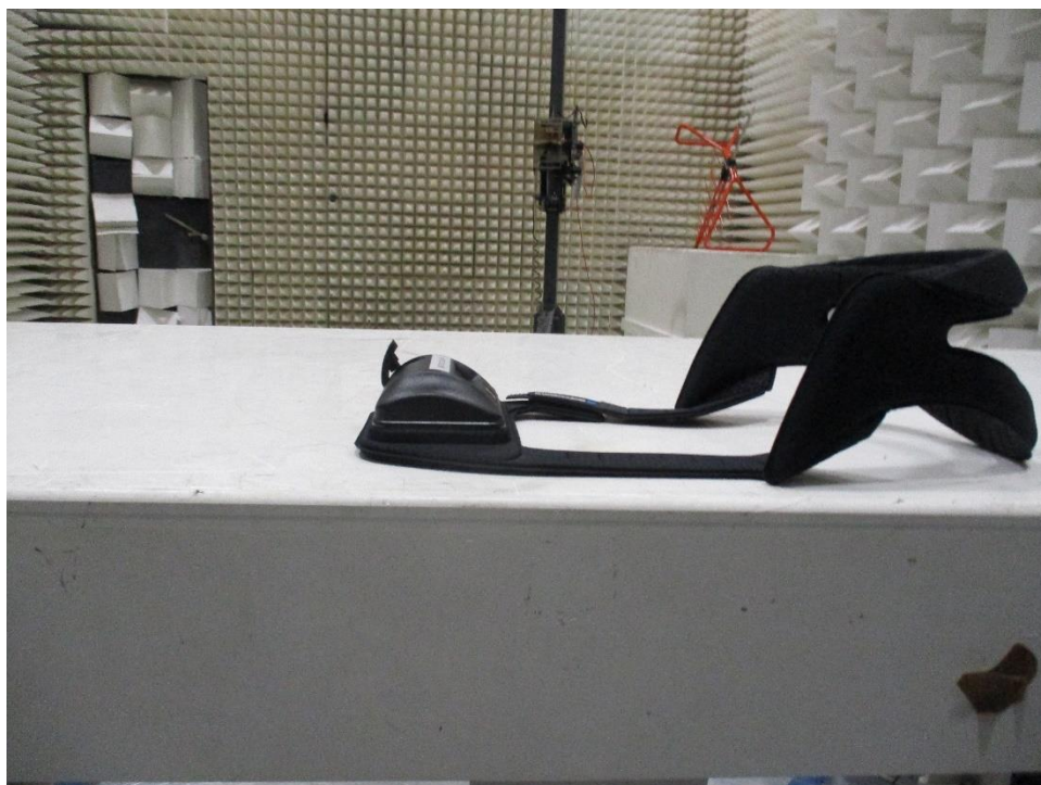
Figure 0-8 Radiated Emissions Test Setup Above 1 GHz Battery Mode Back Side
