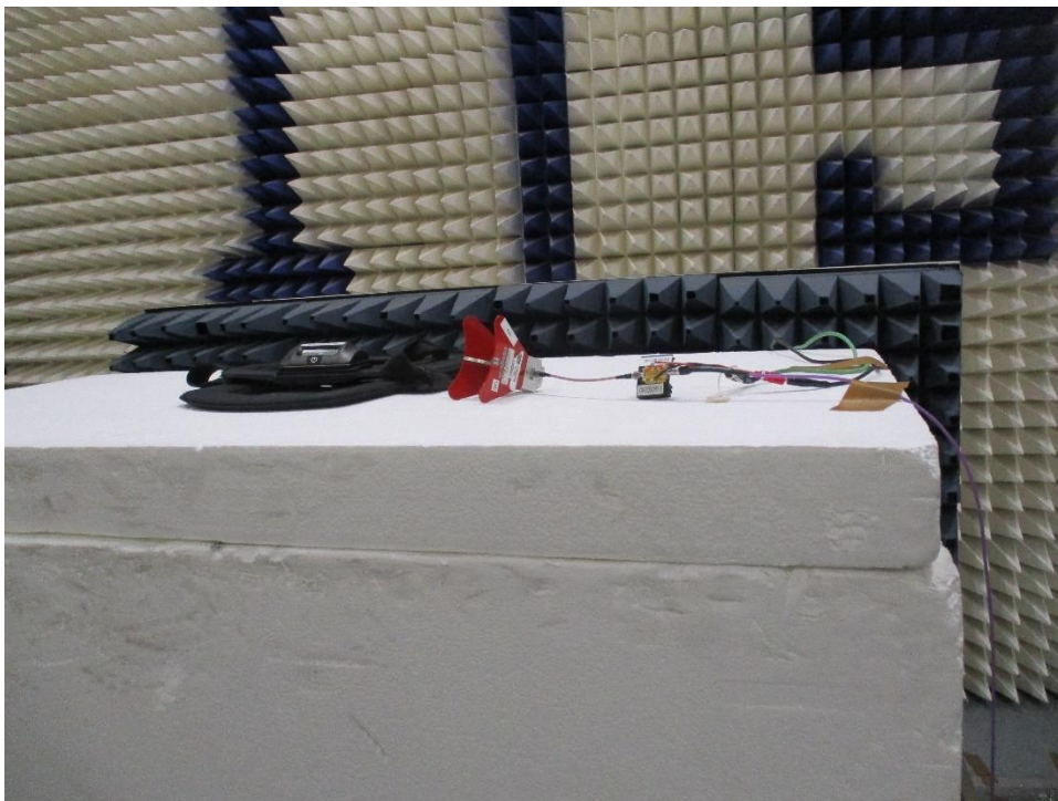
Figure 0-34 Radiated Spurious Emissions Test Setup Above 18 GHz Battery Mode
