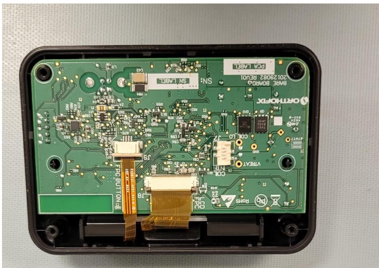
Figure 3 - 5212CM Control Module, Cover Removed
