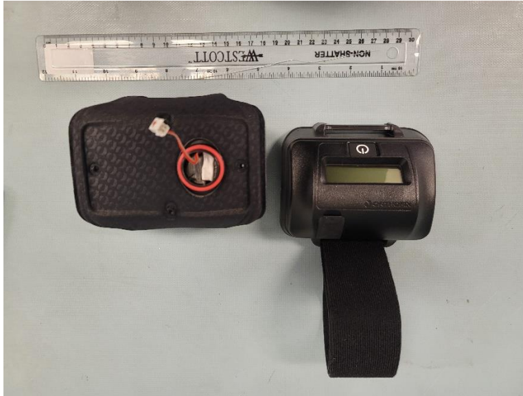
Figure 17 – 5302CM Treatment Coil Removed
