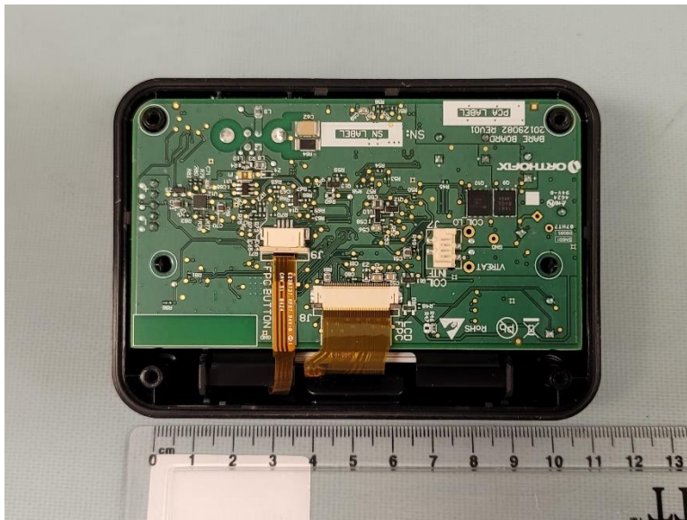
Figure 11 - 5505CM Control Module, Cover Removed
