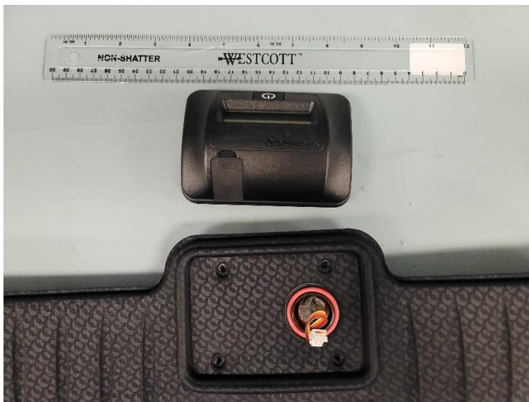
Figure 57 – 5315CM Treatment Coil Removed
