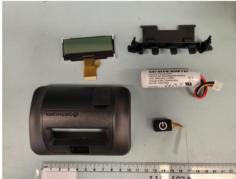
Figure 37 - 5313CM Control Module, All Components Removed
