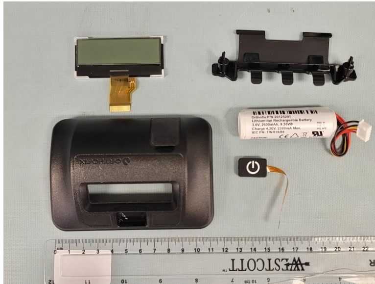
Figure 13 - 5505CM Control Module, All Components Removed
