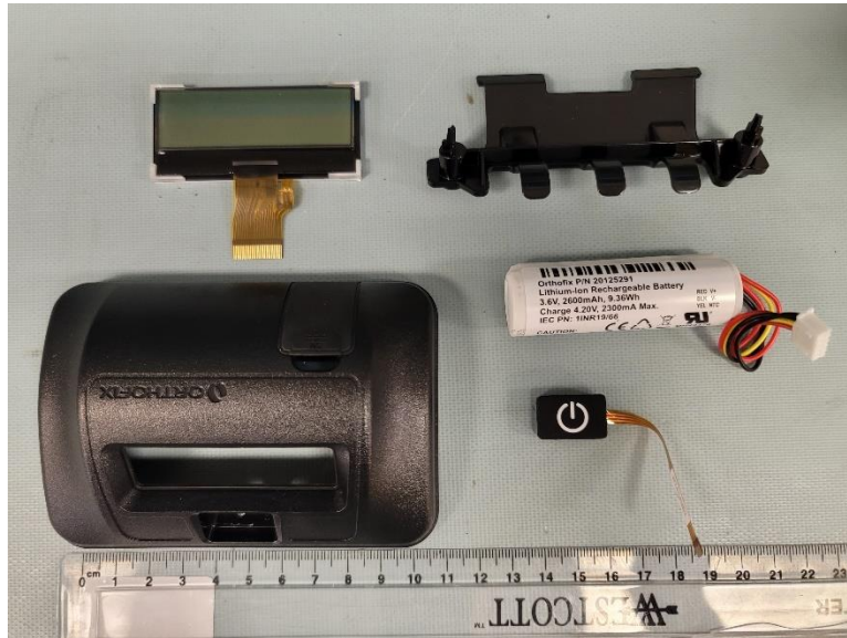
Figure 29 - 5303CM Control Module, All Components Removed
