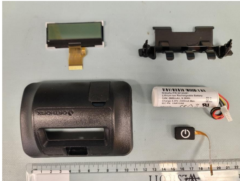
Figure 45 - 5314RCM Control Module, All Components Removed
