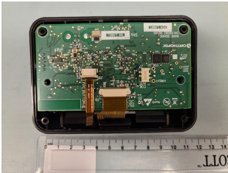
Figure 35 - 5313CM Control Module, Cover Removed
