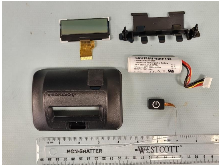
Figure 5 - 5212CM Control Module, All Components Removed
