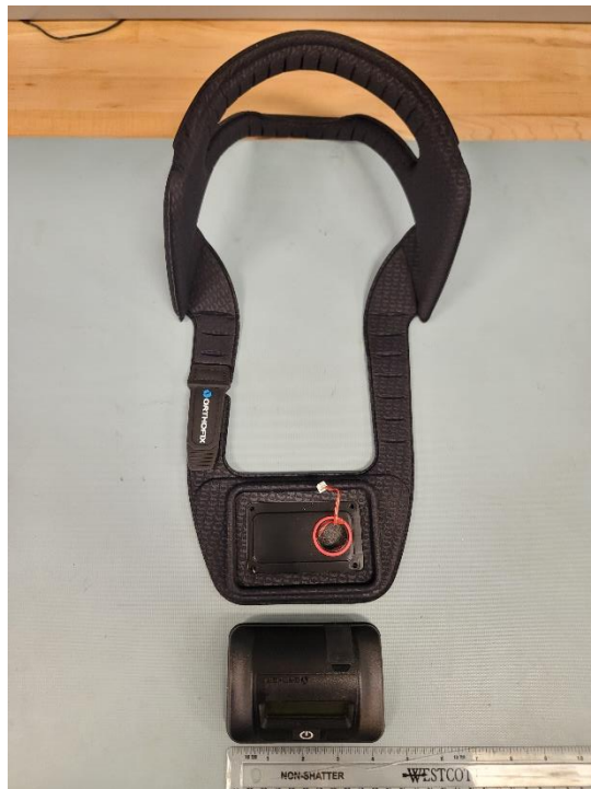
Figure 9 – 5505CM Treatment Coil Removed
