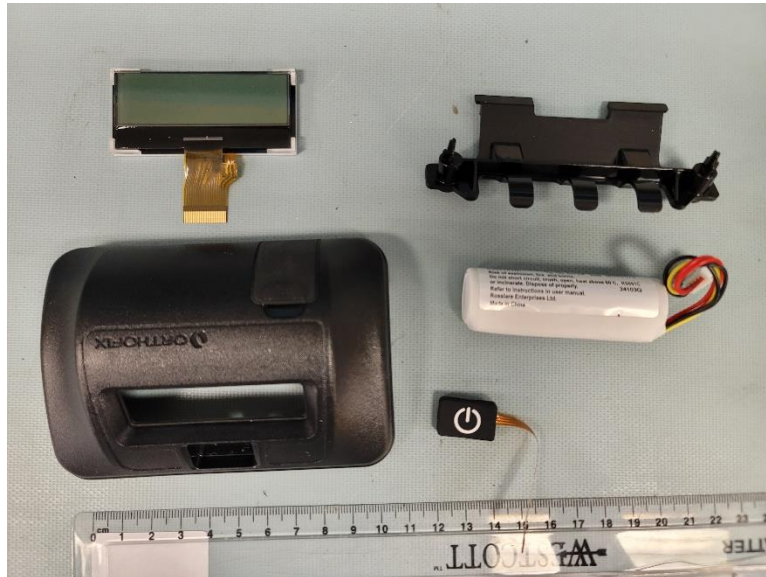
Figure 61 - 5315CM Control Module, All Components Removed
