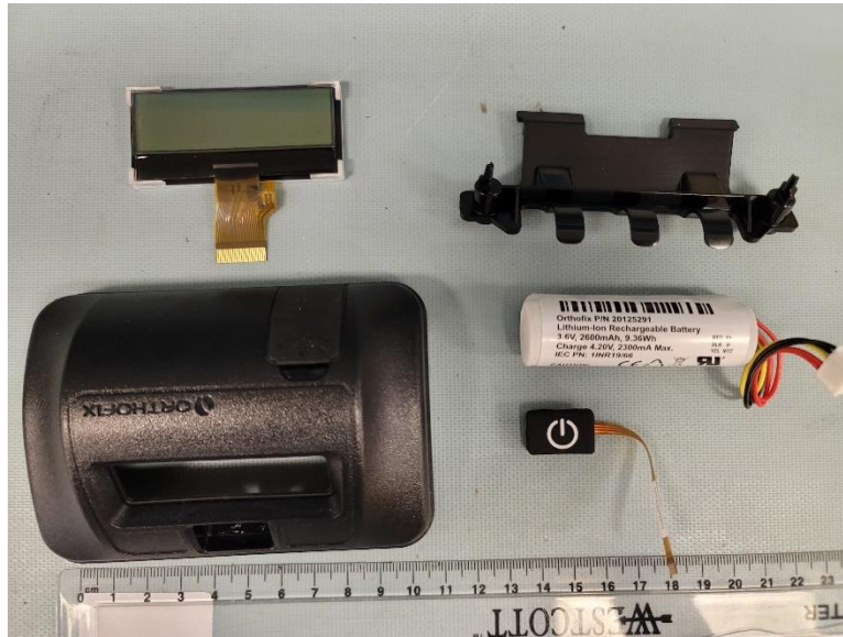
Figure 53 - 5314LCM Control Module, All Components Removed
