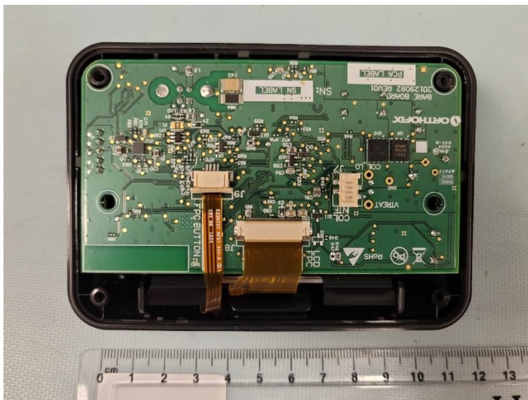
Figure 27 - 5303CM Control Module, Cover Removed
