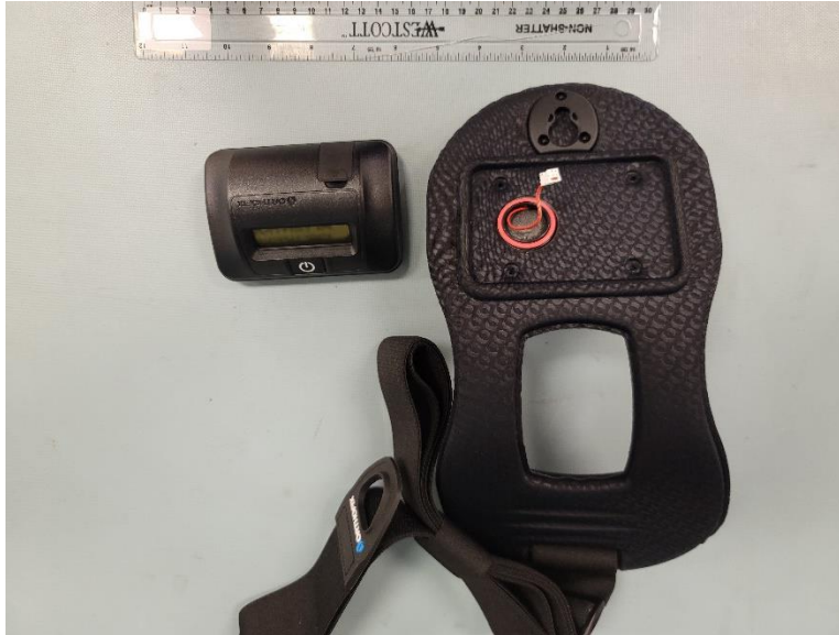
Figure 33 – 5313CM Treatment Coil Removed
