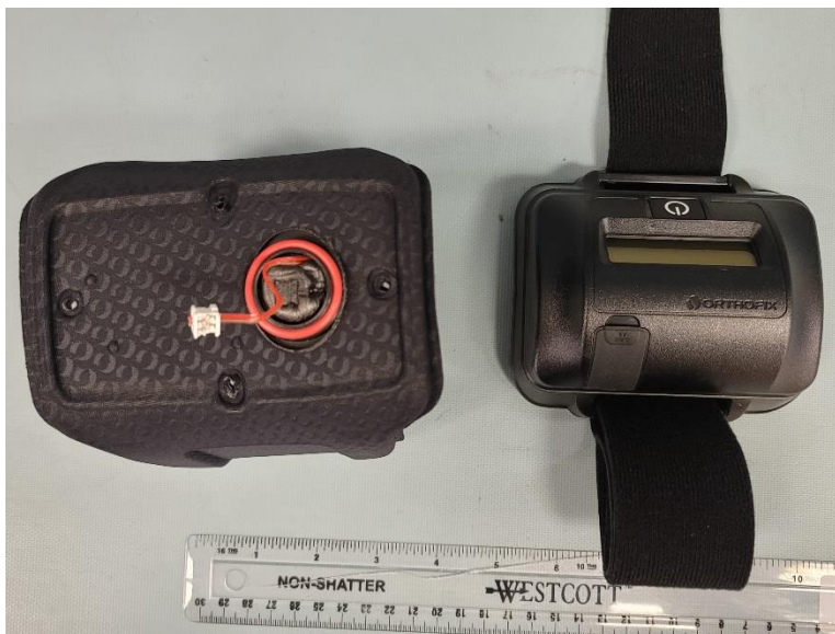
Figure 25 – 5303CM Treatment Coil Removed
