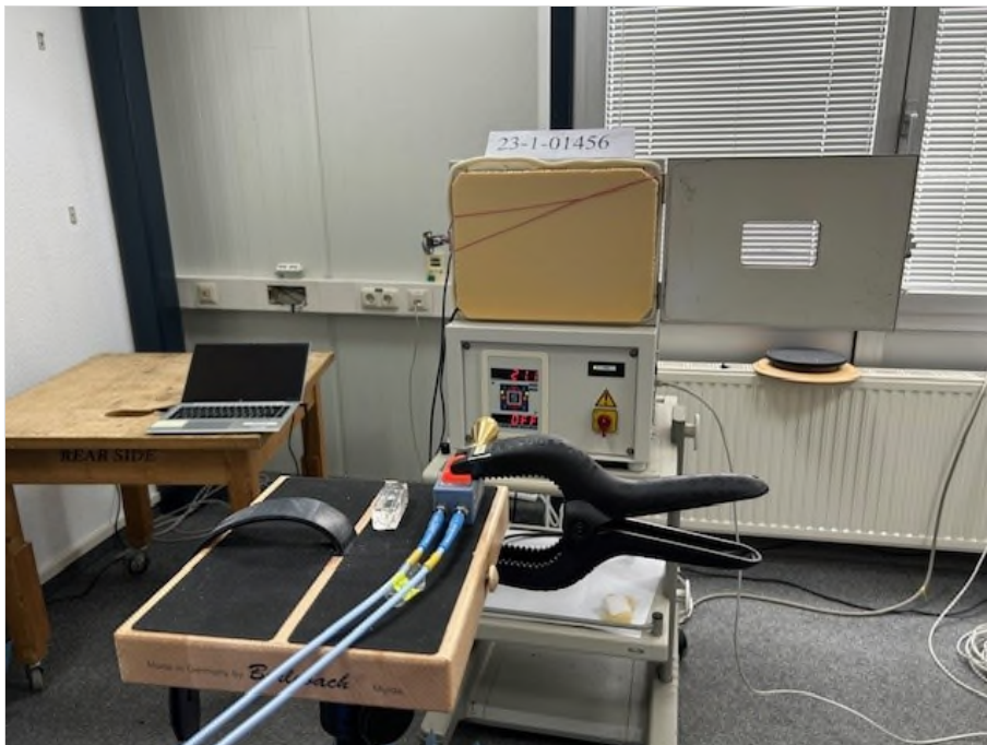
Photograph 10: EUT test setup in the semi anechoic chamber, overview_EUT
