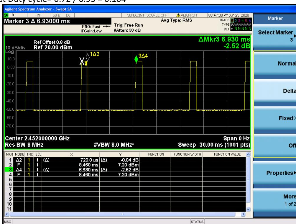
Calculating the AV value according to the duty cycle
