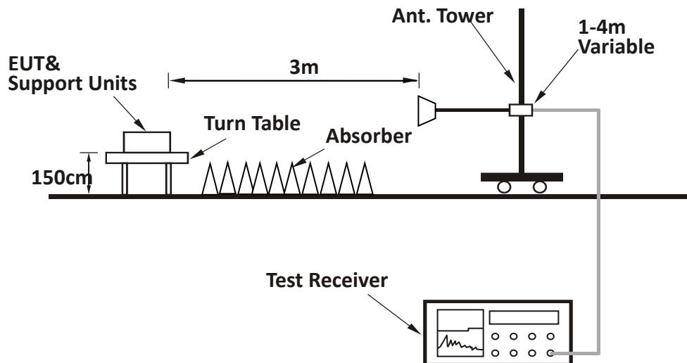
**TEST REPORT****3.4 Test Results of Radiated Emissions**
