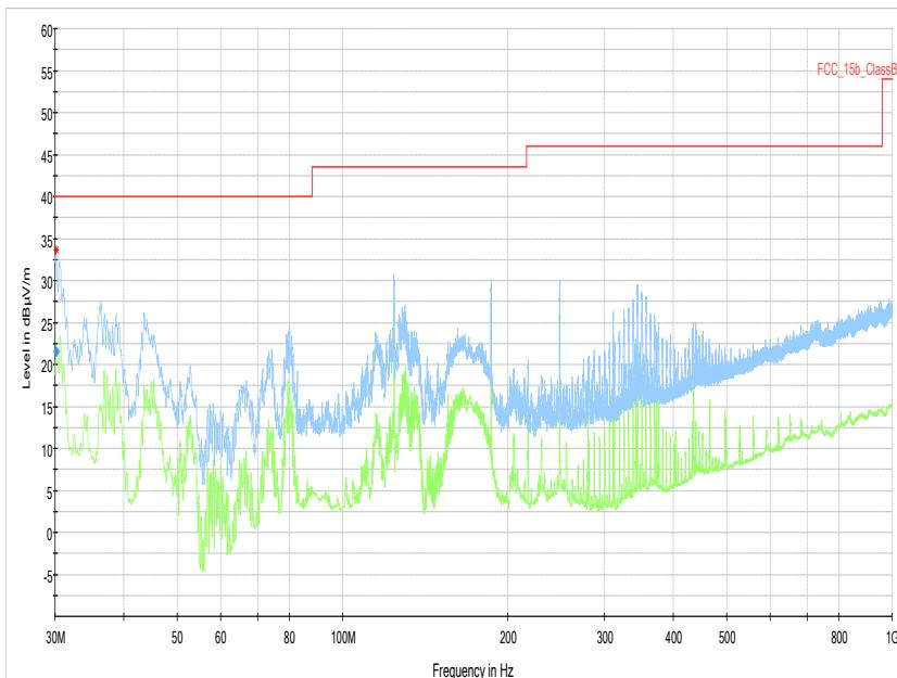
AC mains connection = via connected computer device, Measurement range = 30 MHz - 1 GHz, Test setup = computer peripheral
