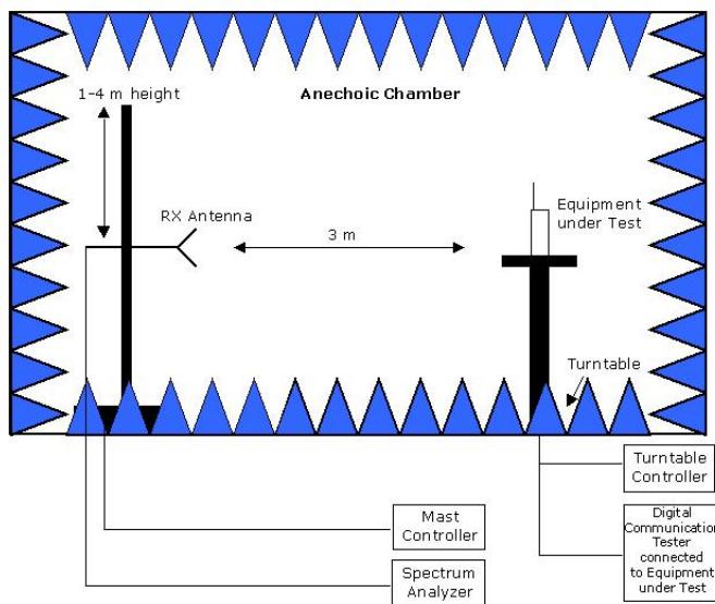
Setup in the Anechoic chamber. For measurements below 1 GHz the ground was replaced by a conducting ground plane.
