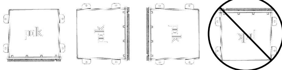
2. Using the shortest length of the recommended size screws possible, mount the tuner/ amplifier as detailed in the diagram to the right.
