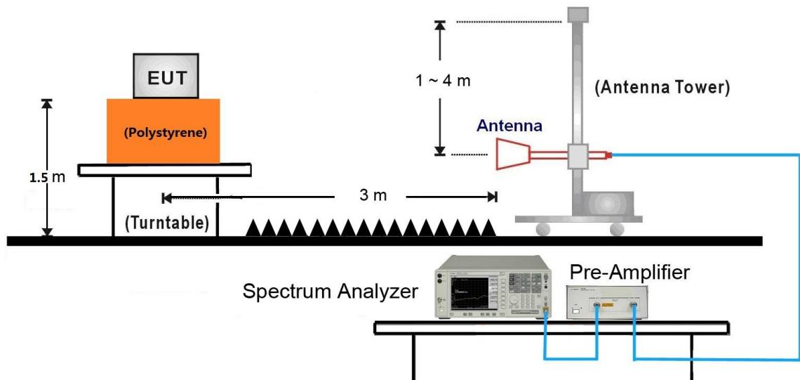
18GHz ~25GHz Test Setup:
