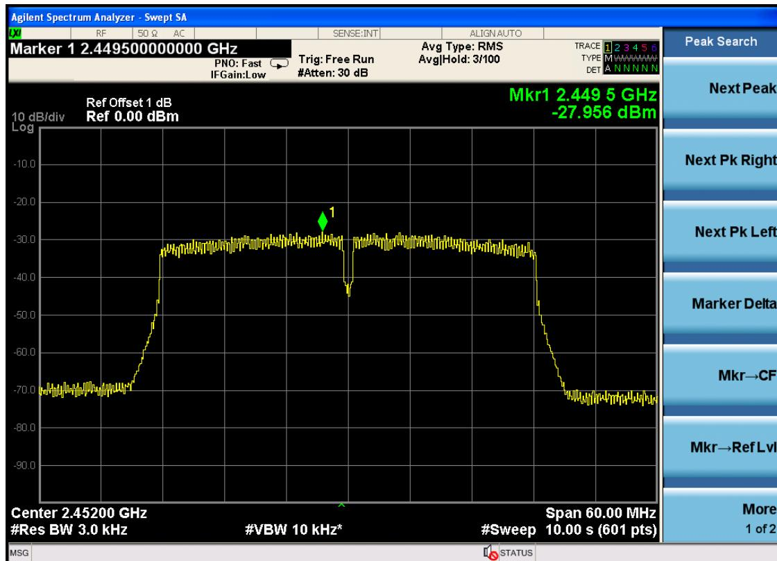
**For MIMO antenna port 1+antenna port 2**
