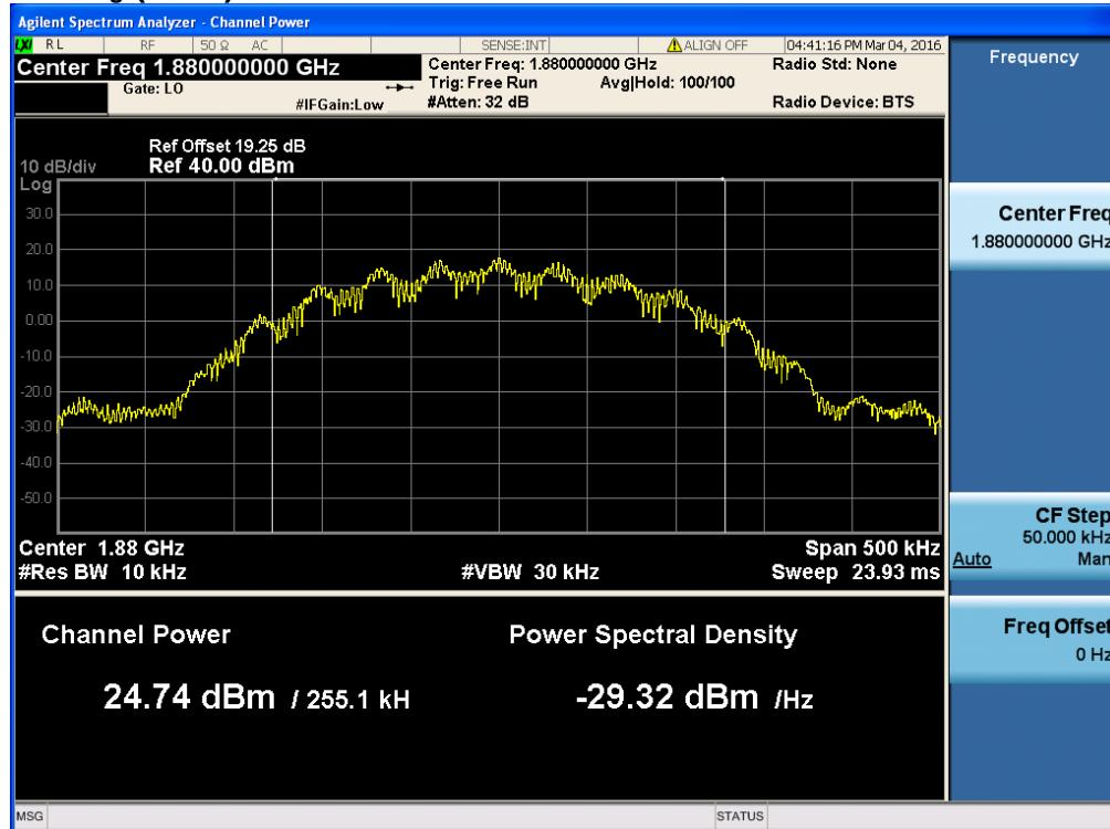
$$\text{PAR (dB)} = P_{Pk} (\text{dBm}) - P_{Avg} (\text{dBm}) = 28.10 \text{ dBm} - 24.74 \text{ dBm} = 3.36 \text{ dB}$$
