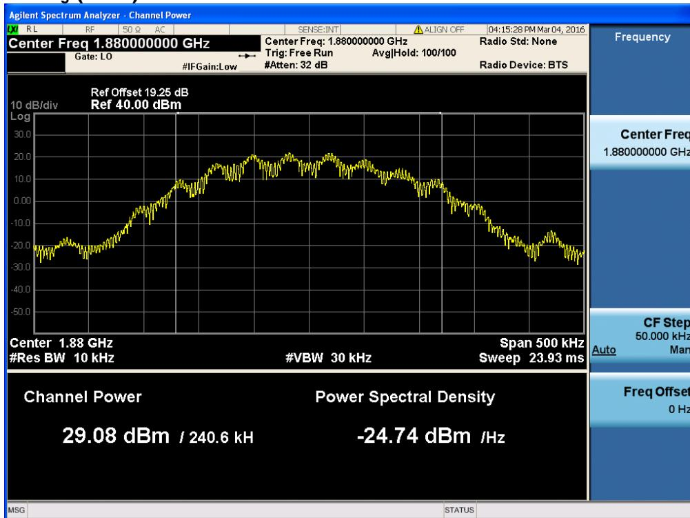
$$\text{PAPR (dB)} = \text{P}_{\text{Pk}} (\text{dBm}) - \text{P}_{\text{Avg}} (\text{dBm}) = 29.62 \text{ dBm} - 29.08 \text{ dBm} = 0.54 \text{ dB}$$
