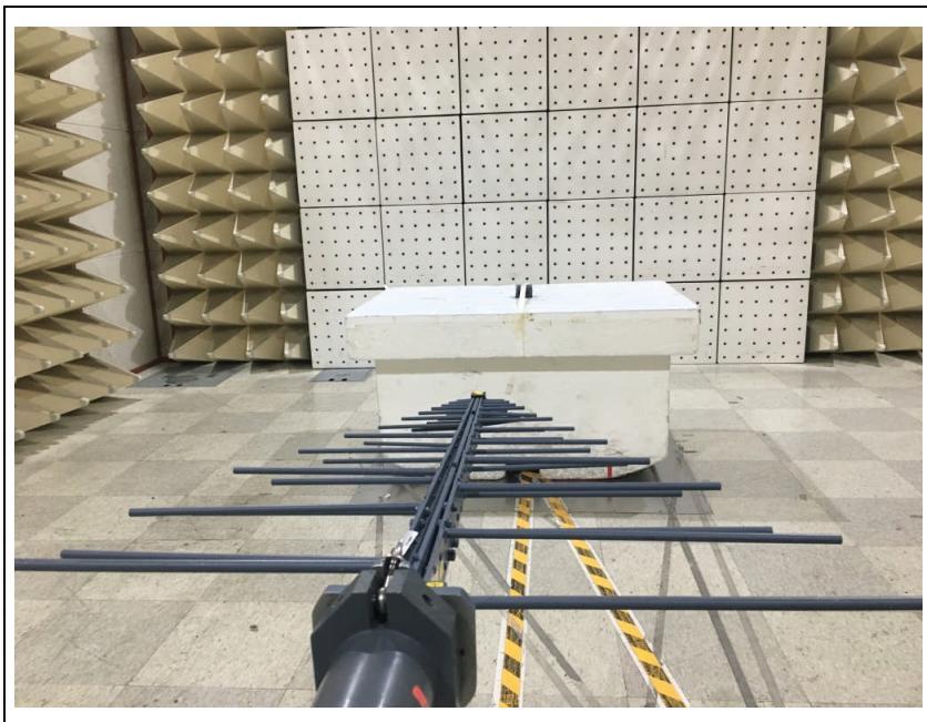
**3. Photo of Radiated Spurious Emission Test (Above 1 GHz)**
