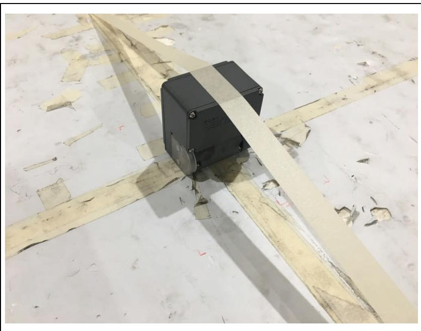
**2. Photo of Radiated Spurious Emission Test (Below 1 GHz)**
