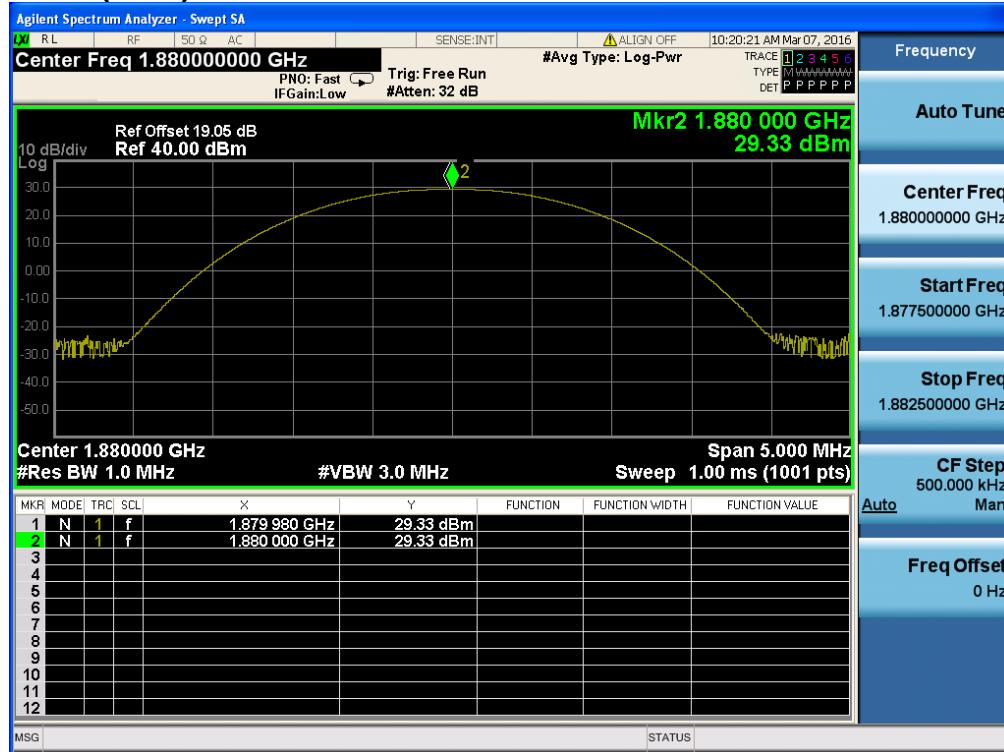
**-P<sub>Avg</sub> (dBm)**      GPRS 1900 & Channel: 661
