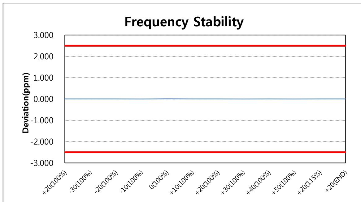
**Note.** Based on the results of the frequency stability test at the center channel the frequency deviation results measured are very small. as such it is determined that the channels at the band edge would remain inband when the maximum measured frequency deviation noted during the frequency stability tests is applied. therefore the device is determined to remain operating in band over the temperature and voltage range as tested.
