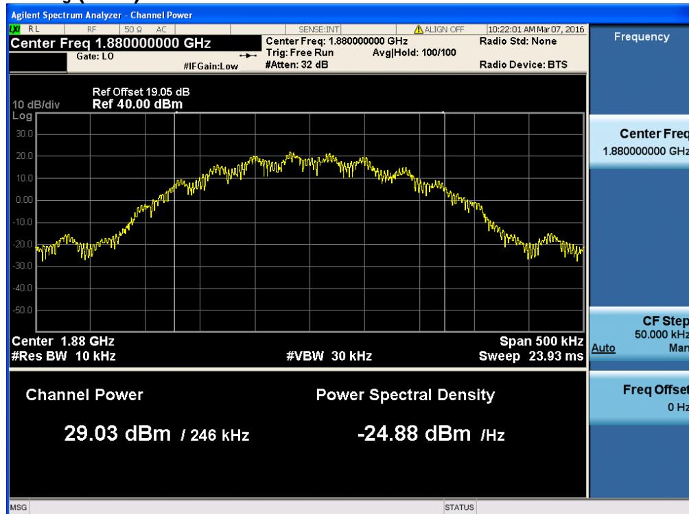
$$\text{PAPR (dB)} = \text{P}_{\text{Pk}} (\text{dBm}) - \text{P}_{\text{Avg}} (\text{dBm}) = 29.33 \text{ dBm} - 29.03 \text{ dBm} = 0.30 \text{ dB}$$
