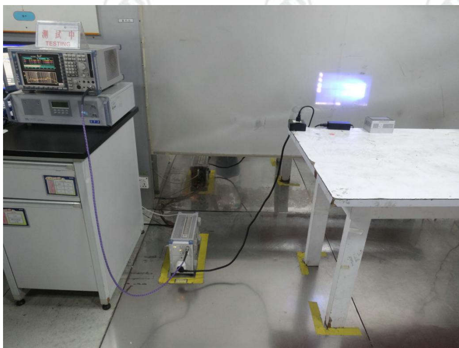
Conducted Emissions Test Setup
