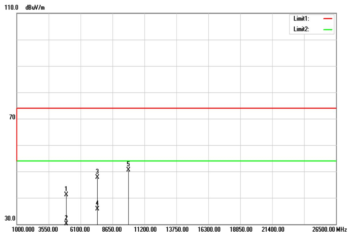
**Operation Mode:** GFSK / TX / CH High**Test Date:** May 13, 2016**Temperature:** 27°C**Tested by:** Jason Lu**Humidity:** 53 % RH**Polarity:** Ver. / Hor.
