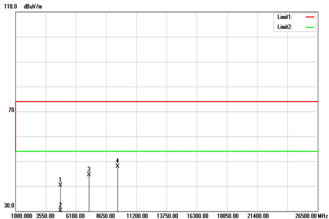
**Above 1 GHz****Operation Mode:** GFSK / TX / CH Low**Test Date:** May 13, 2016**Temperature:** 27°C**Tested by:** Jason Lu**Humidity:** 53 % RH**Polarity:** Ver. / Hor.
