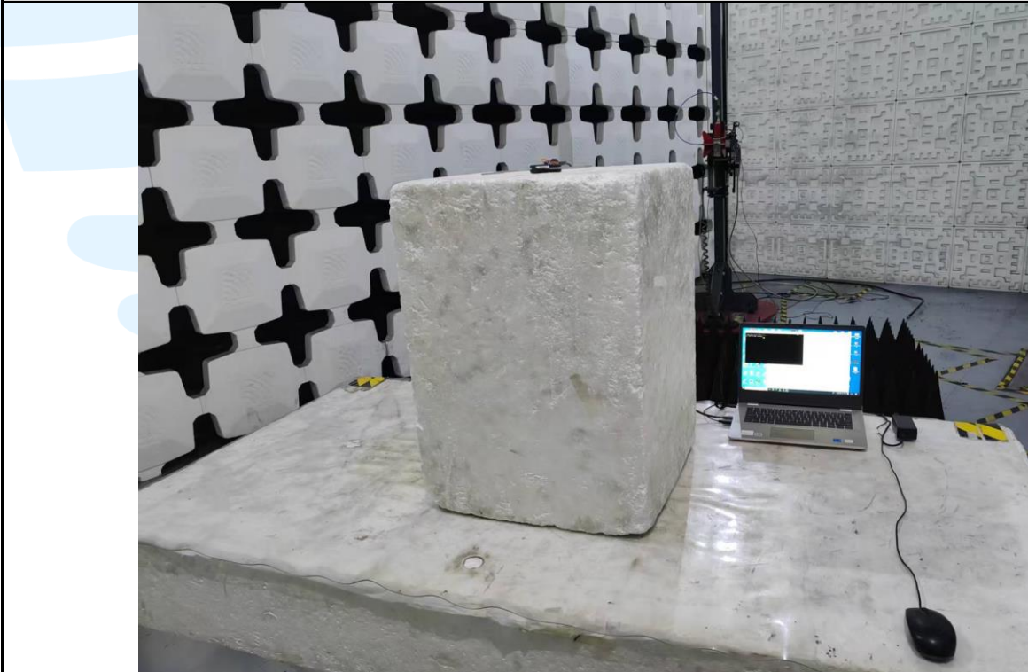
Radiated emission Test Setup (Above 1 GHz)
