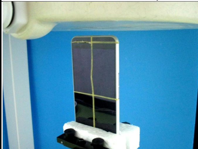
Top Side of EUT with 1.0 cm Gap
