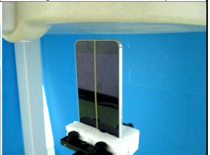
Bottom Side of EUT with 1.0 cm Gap
