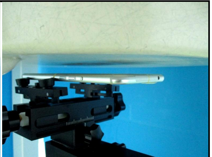
Rear Face of EUT with 1.0 cm Gap
