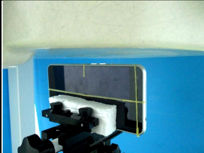
Left Side of EUT with 1.0 cm Gap
