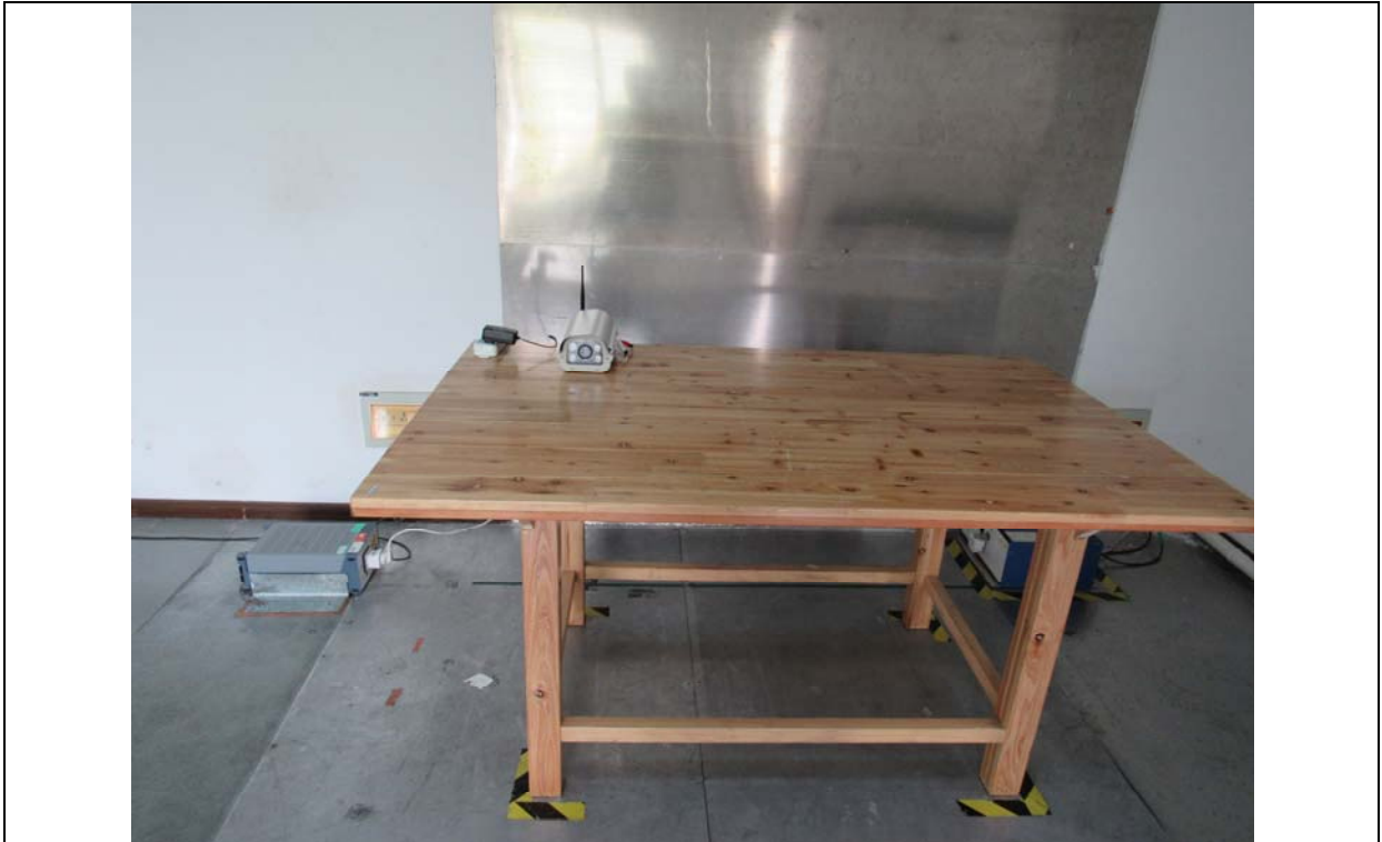
Conducted Emissions Setup Front View
