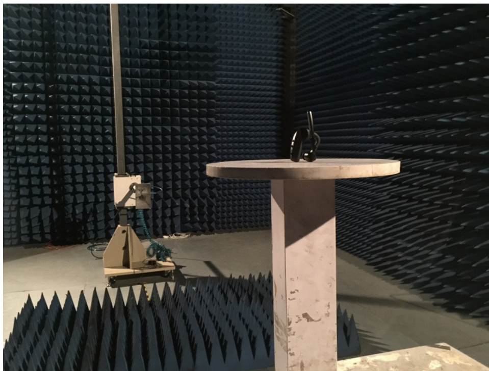
Setup for Radiated Emission
