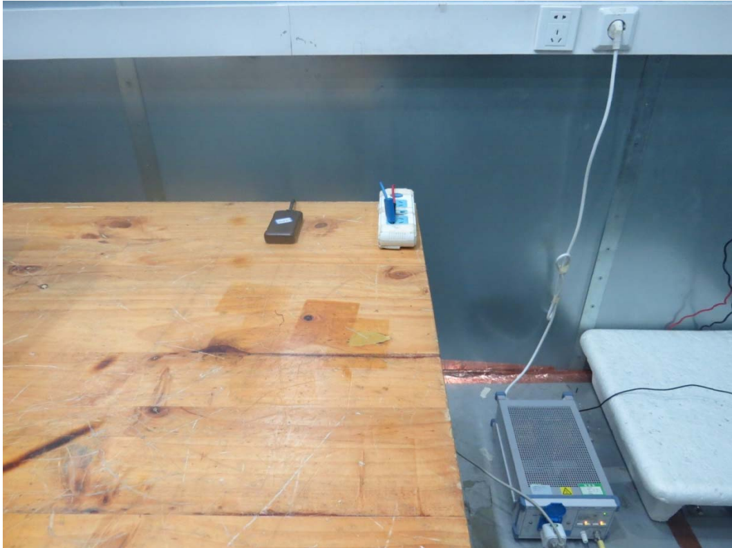
Picture 2 Conducted Emission Test Setup
