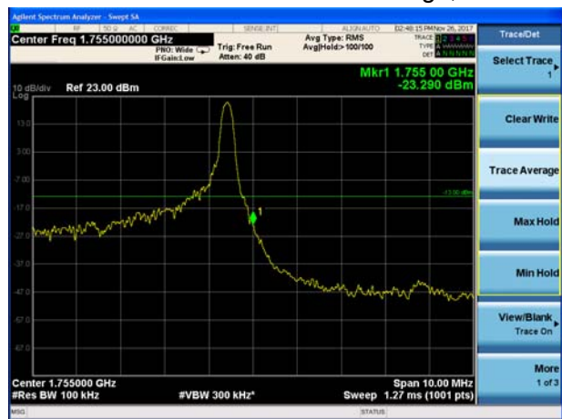
LTE Band 4 QPSK 10MHz CH-High, 1 RB
