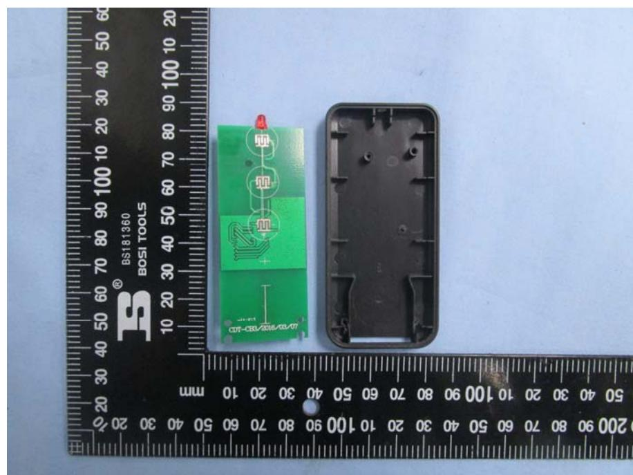
**Solder Board-Component View 1**
