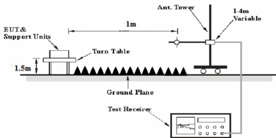
The radiated emission Below 1GHz tests were performed in the 3 meters chamber test site A, above 1GHz tests were performed in the 3 meters chamber test site B, using the setup accordance with the ANSI C63.10-2013. The specification used was the FCC 15.209, and FCC 15.407 limits.
