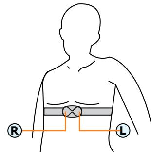
The induction belt wear on slightly below chest. Put the i-Heart onto central of body and determine is it close to your skin
