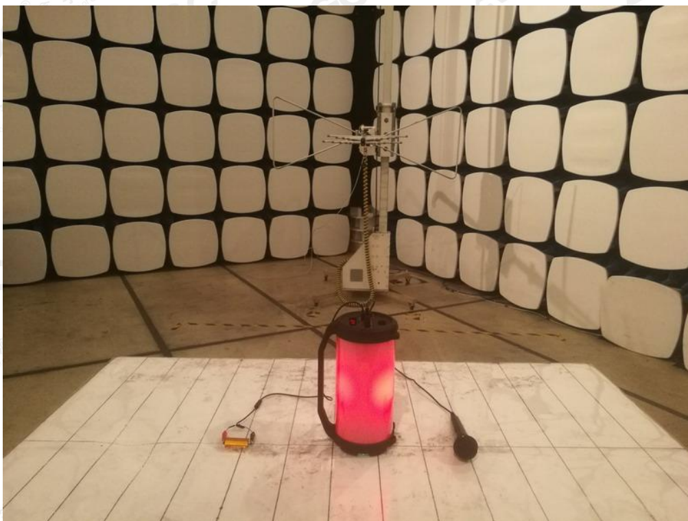
FCC RADIATED EMISSION TEST SETUP
