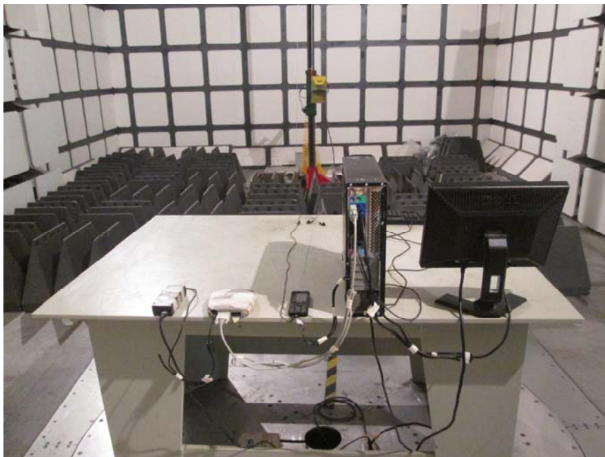
Radiated Emissions – Rear View (Above 1 GHz)
