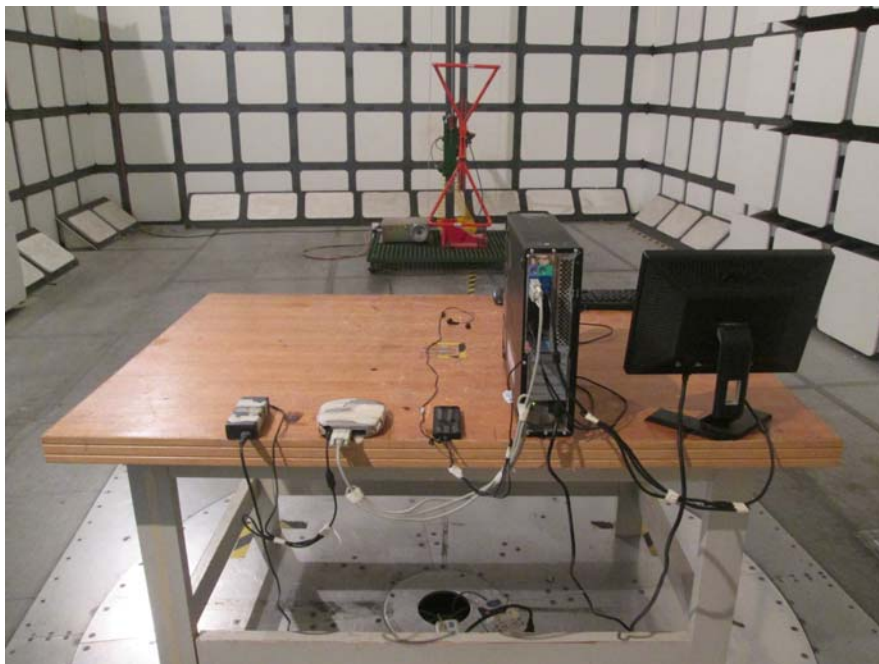
Radiated Emissions – Rear View (Below 1 GHz)
