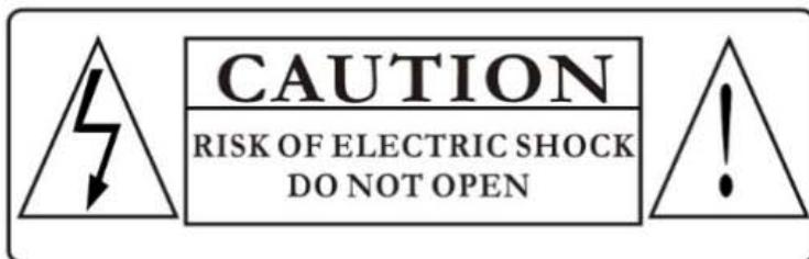
The symbols shown above are internationally accepted symbols that warn of potential hazards with electrical products. The lightning flash with arrow point in an equilateral triangle means that there are dangerous voltages present within the unit. The exclamation point in an equilateral triangle indicates that it is necessary for the user to refer to the owner's manual.
