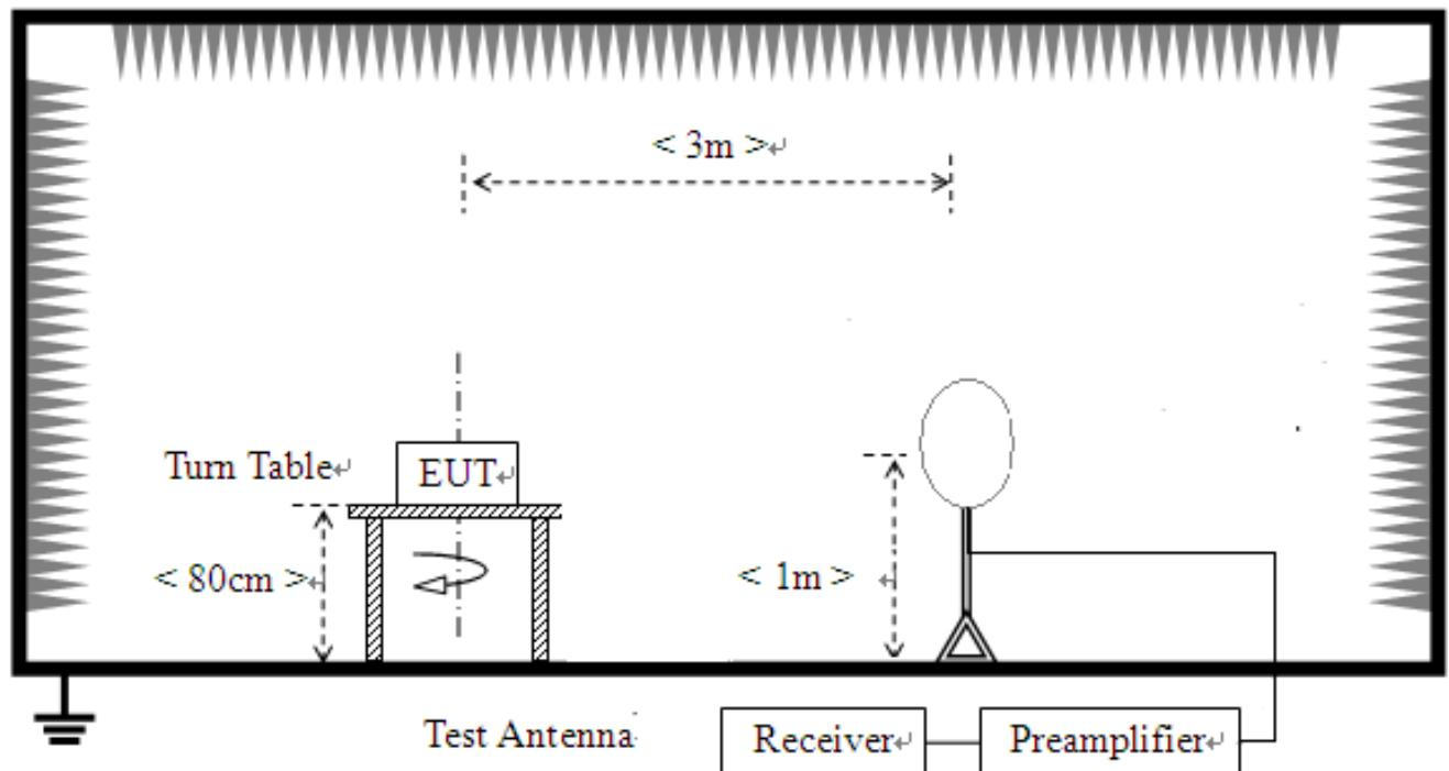
For radiated emissions from 30MHz to 1GHz
