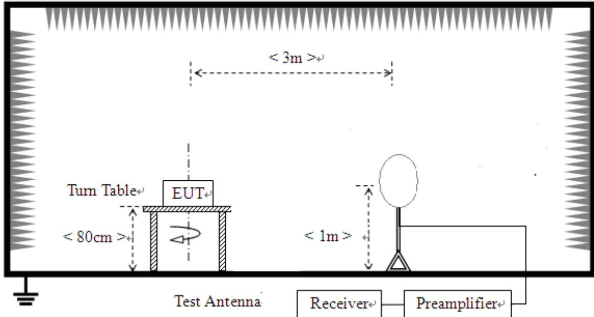
For radiated emissions from 30MHz to 1GHz
