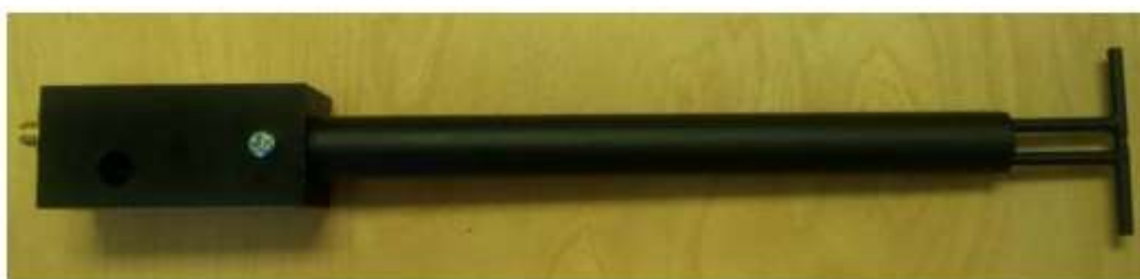
Figure 1 – MVG COMOSAR Validation Dipole
