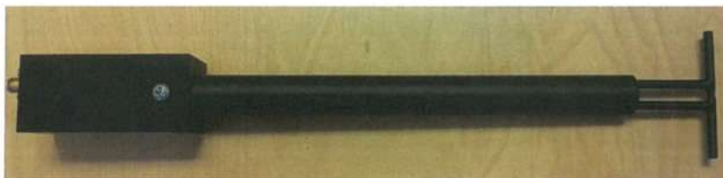
Figure 1 – MVG COMOSAR Validation Dipole
