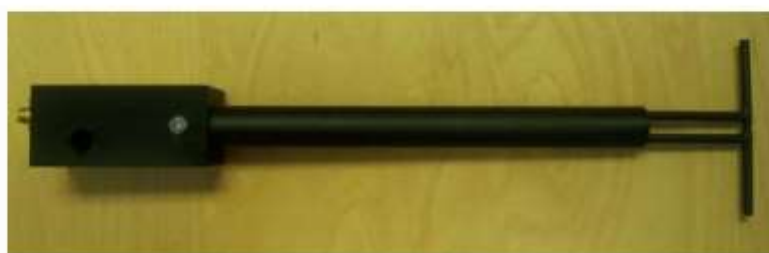
Figure 1 – MVG COMOSAR Validation Dipole
