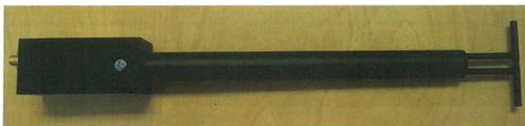
Figure 1 – MVG COMOSAR Validation Dipole
