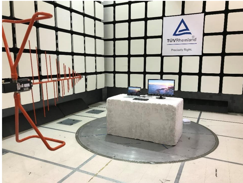
Figure 2: 30 - 1000 MHz Radiated Emissions Test Setup - Front
