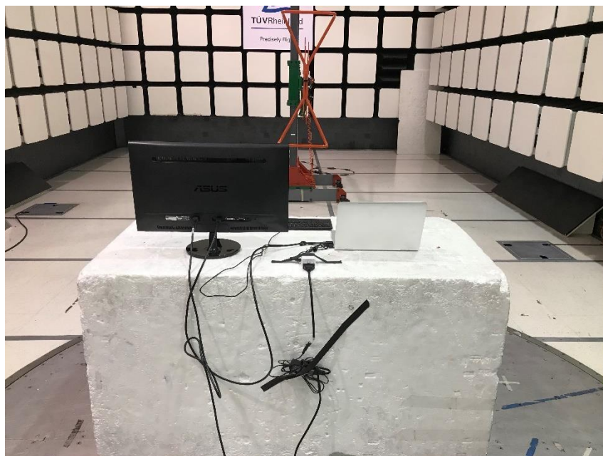
Figure 3: 30 - 1000 MHz Radiated Emissions Test Setup – Back
