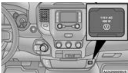
Center Stack Power Inverter
