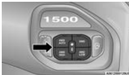
Five-Position/On-Demand Transfer Case — GT Models
