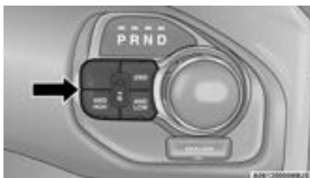
Four-Position/On-Demand Transfer Case
