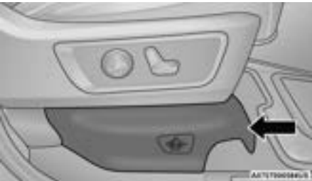
Pull Jack Access Cover From Front
