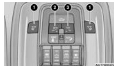
Front Courtesy/Reading Lights
