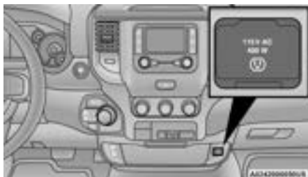
Center Stack Power Inverter
