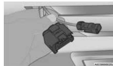
Disconnected Body Side Harness
