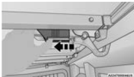
Slide Locking Lever Inward
