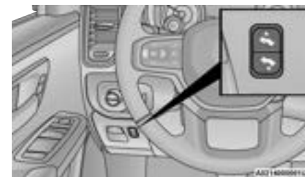
Adjustable Pedals Switch
