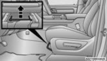
Manual Seat Adjustment Bar
