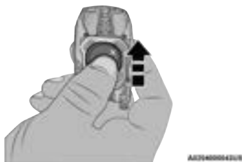
Key Fob Battery Replacement
