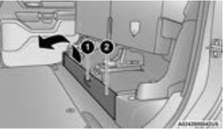
Folding Down Front Of Seat Base
