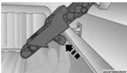
Hold The Bumper And Push The Handle Up
