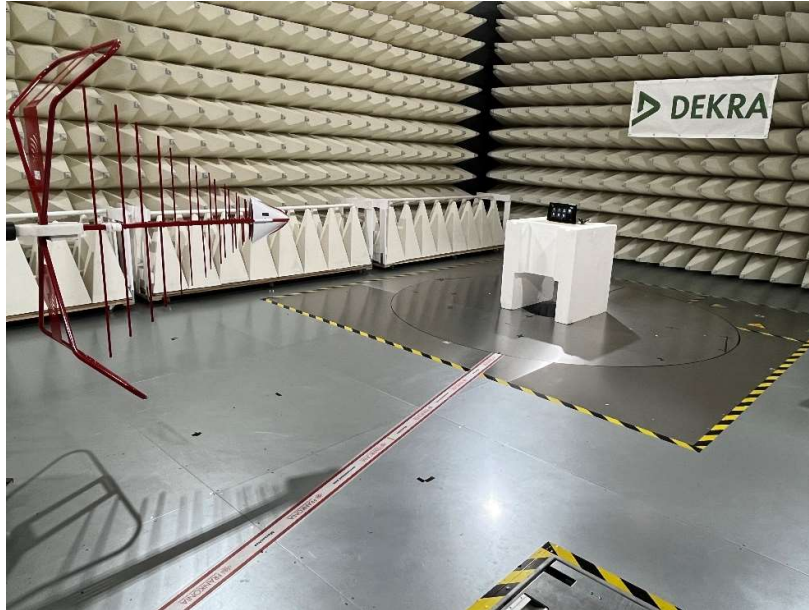
Figure B5. Low Range Radiated Emission test setup
